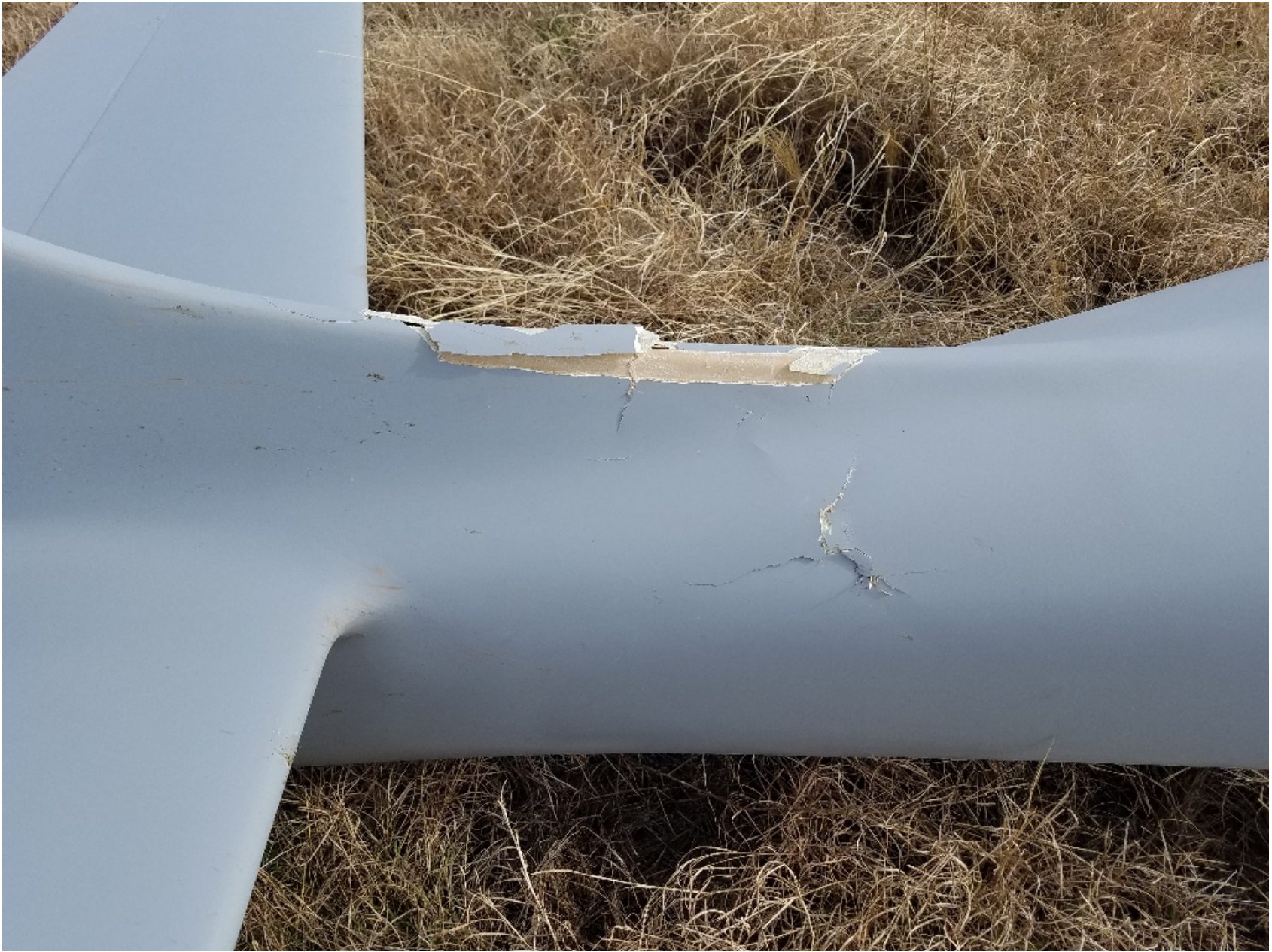
Photo 4 – View of the damage to the fuselage forward of the tail
