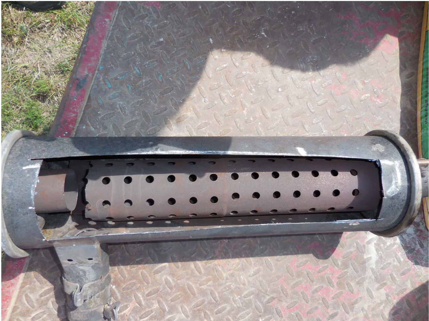
Photo 12 – Heat Exchanger/Muffler Interior Showing Broken Part
