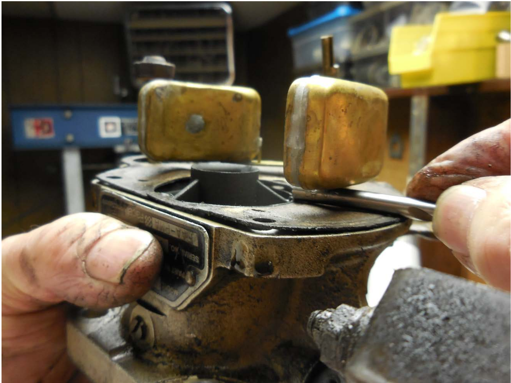
Photo 16 – Carburetor Brass Float and Displacement
