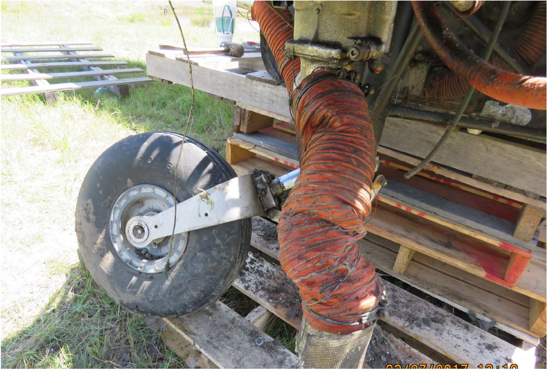
Photo 8 – Scat Host Used for Air Intake Hose to Carburetor
