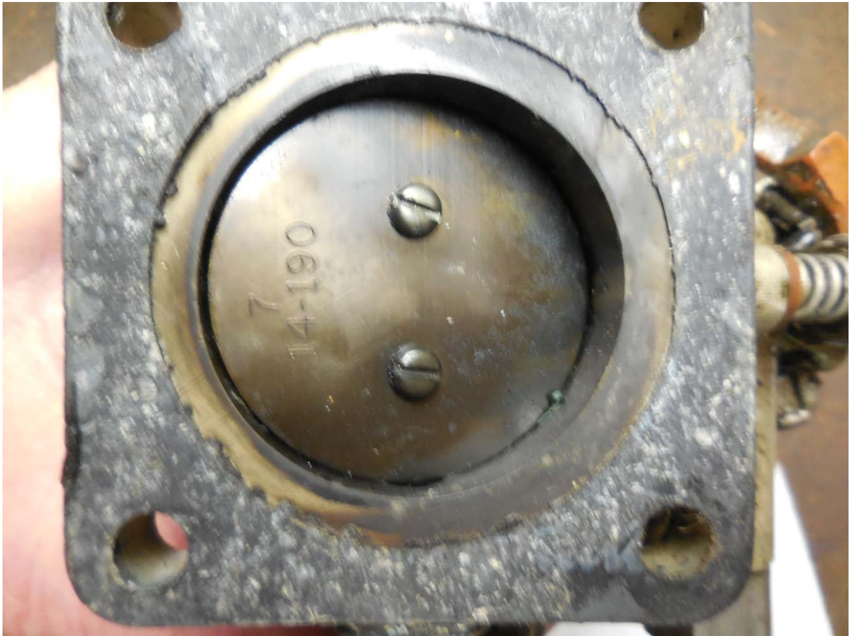
Photo 17 – Carburetor Throttle Valve to Body Gap
