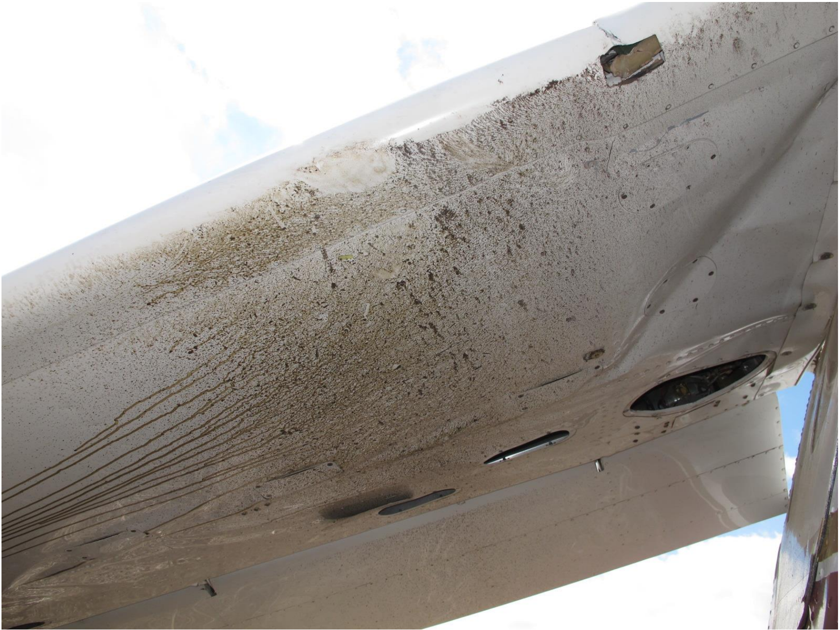
Photo 7 – View of engine oil on the bottom side of the right wing
