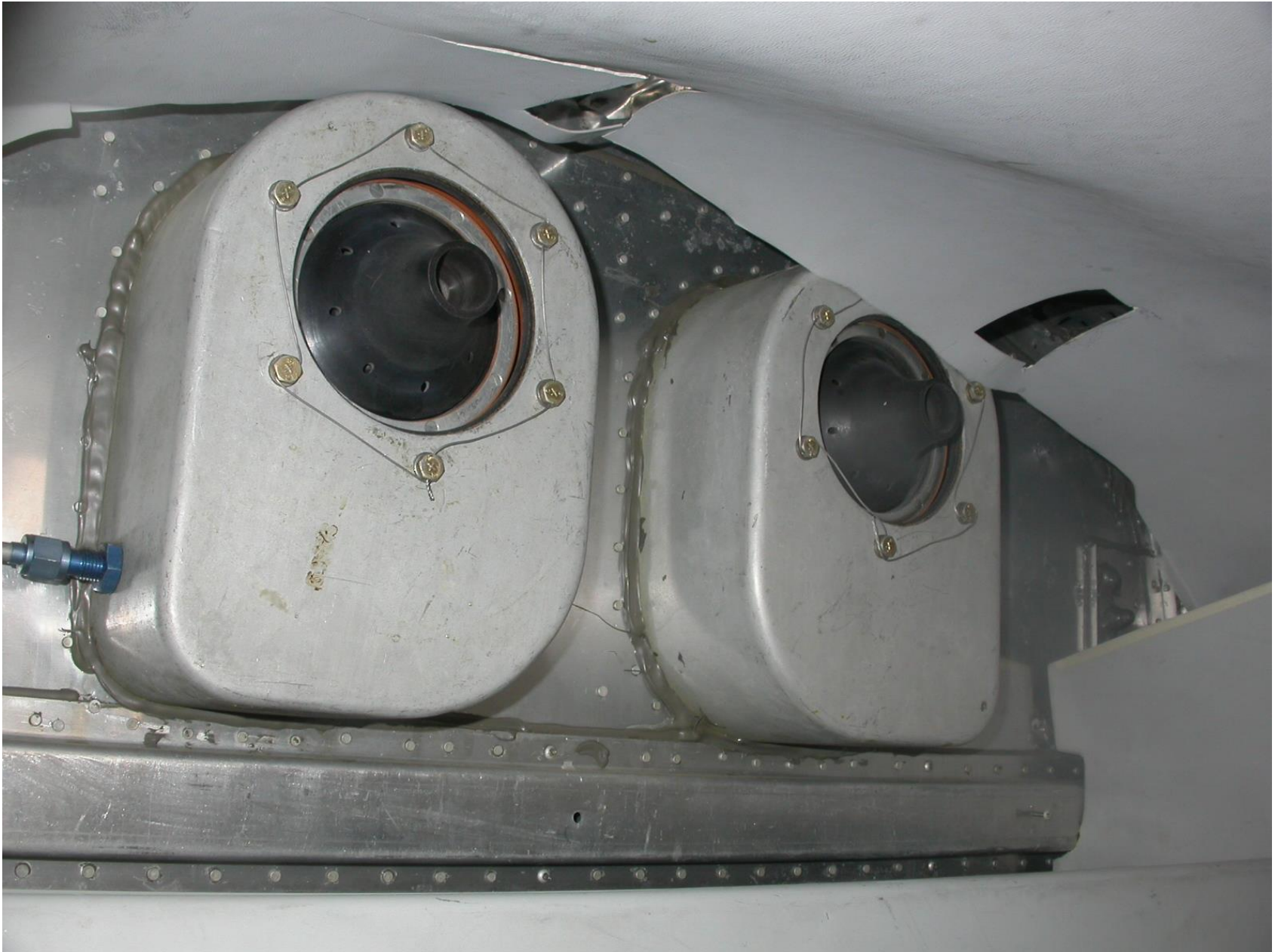
Photo 13 – Cabin Pressurization Dump Valves
