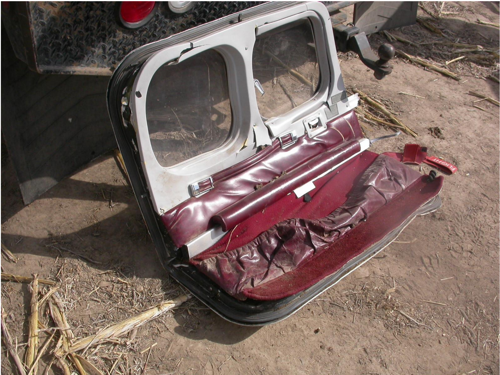
Photo 15 – View of the cabin door and the pressurization seal
