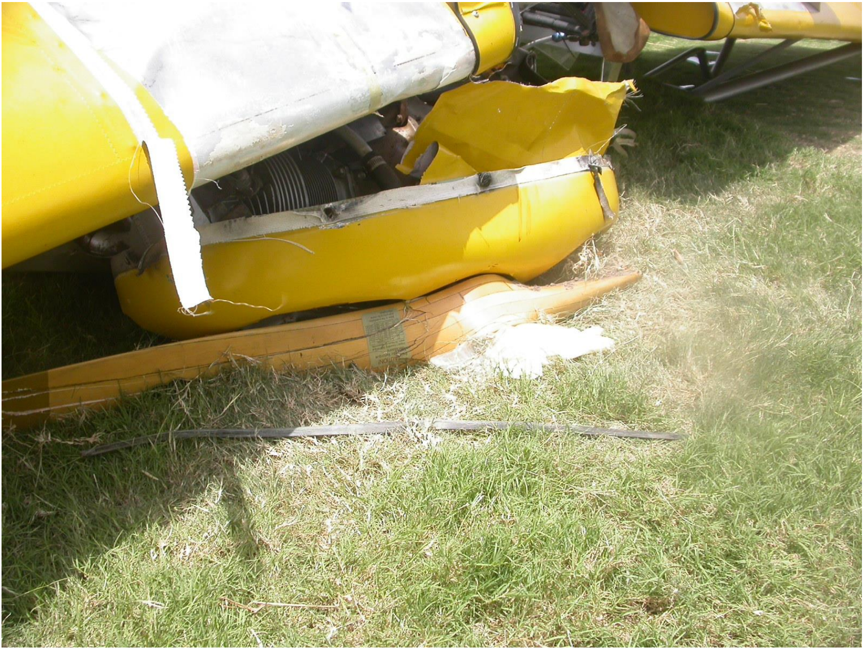
Photo 5 – View of the propeller at the accident site
