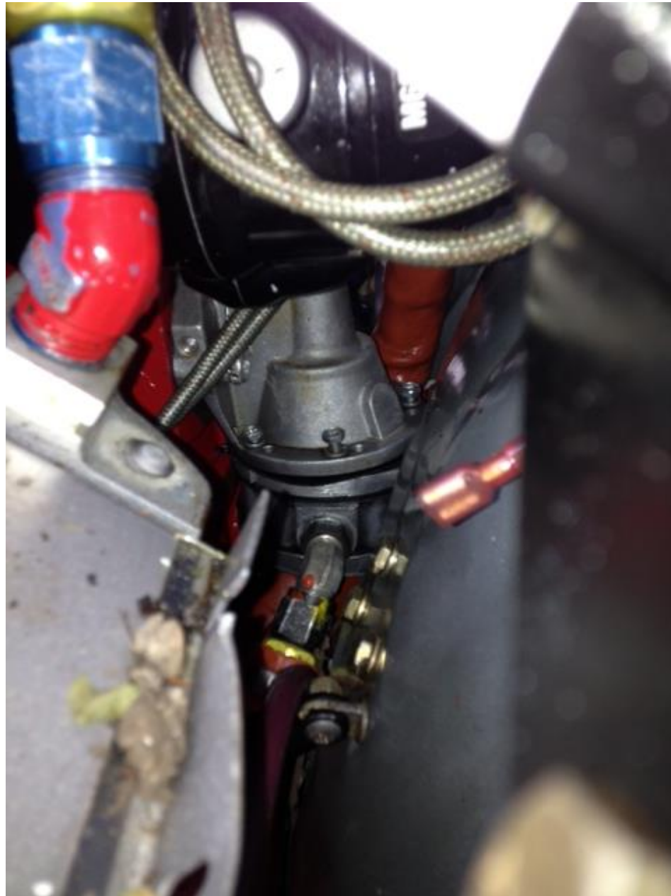
Photo 16 – View of the engine driven fuel pump
