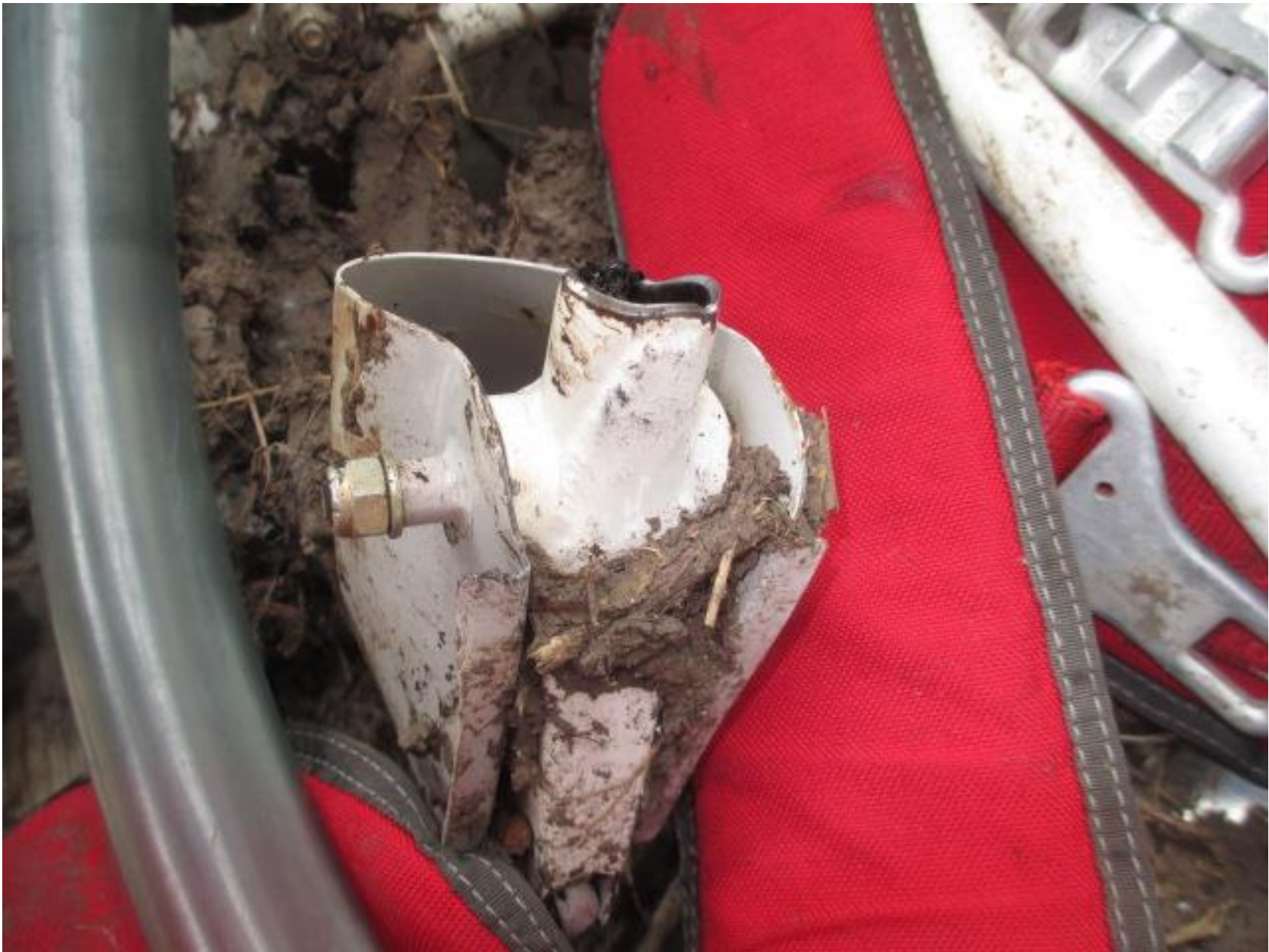
Photo 13 – View of fracture surface of front control stick
