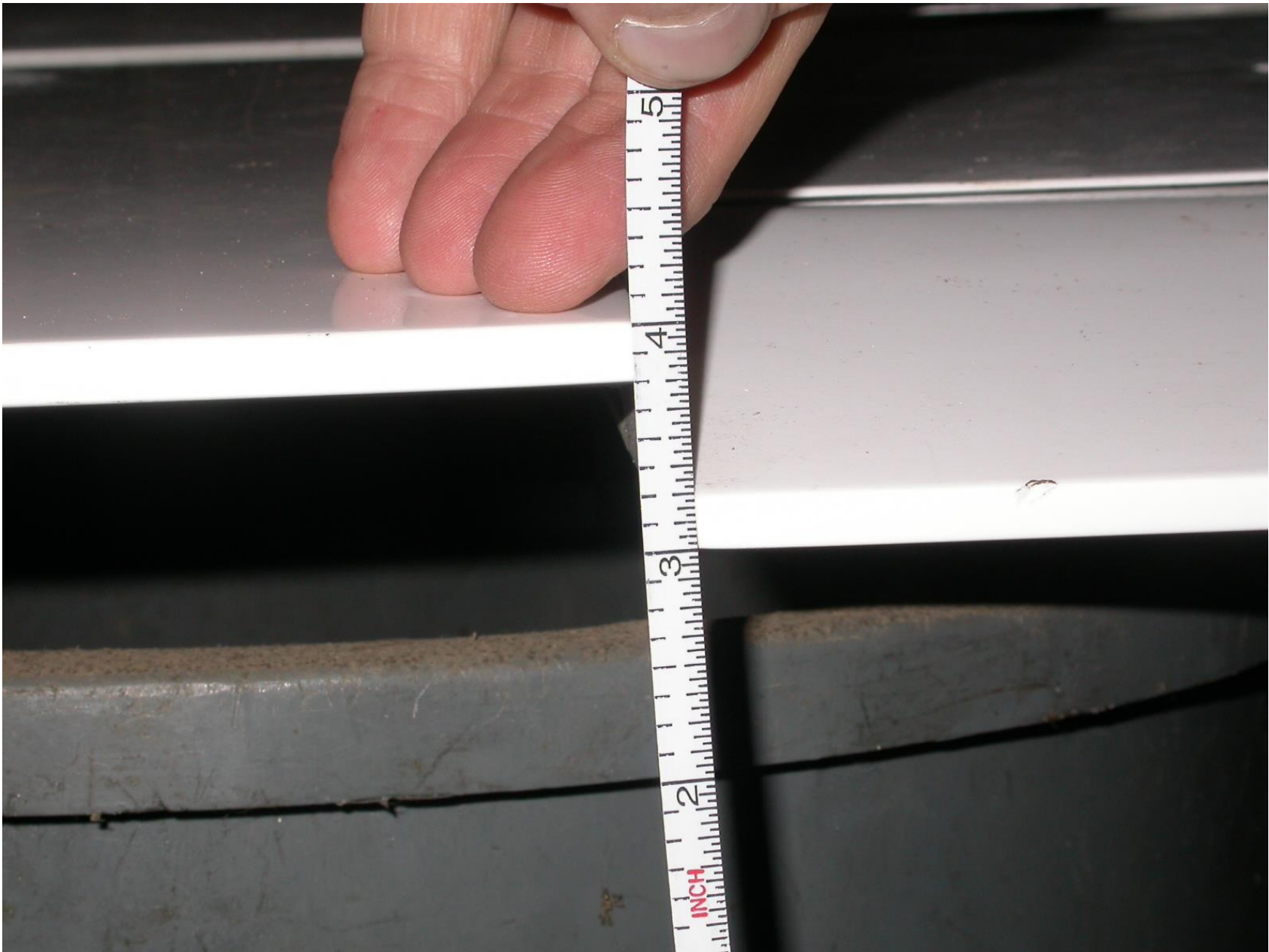
Photo 13 – Rudder Trim Deflection
