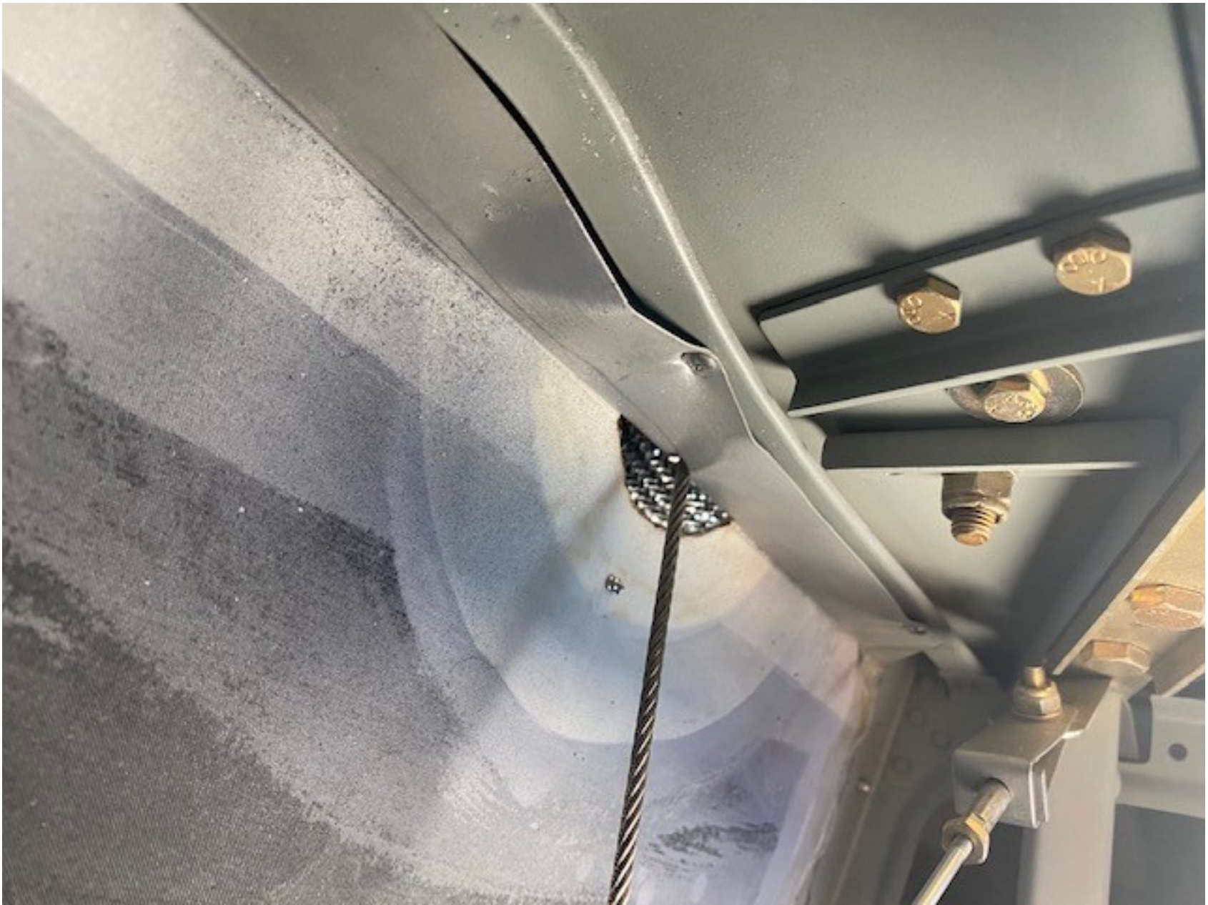
Photo 2 - Damage to the right wing. Photo courtesy of the pilot.
