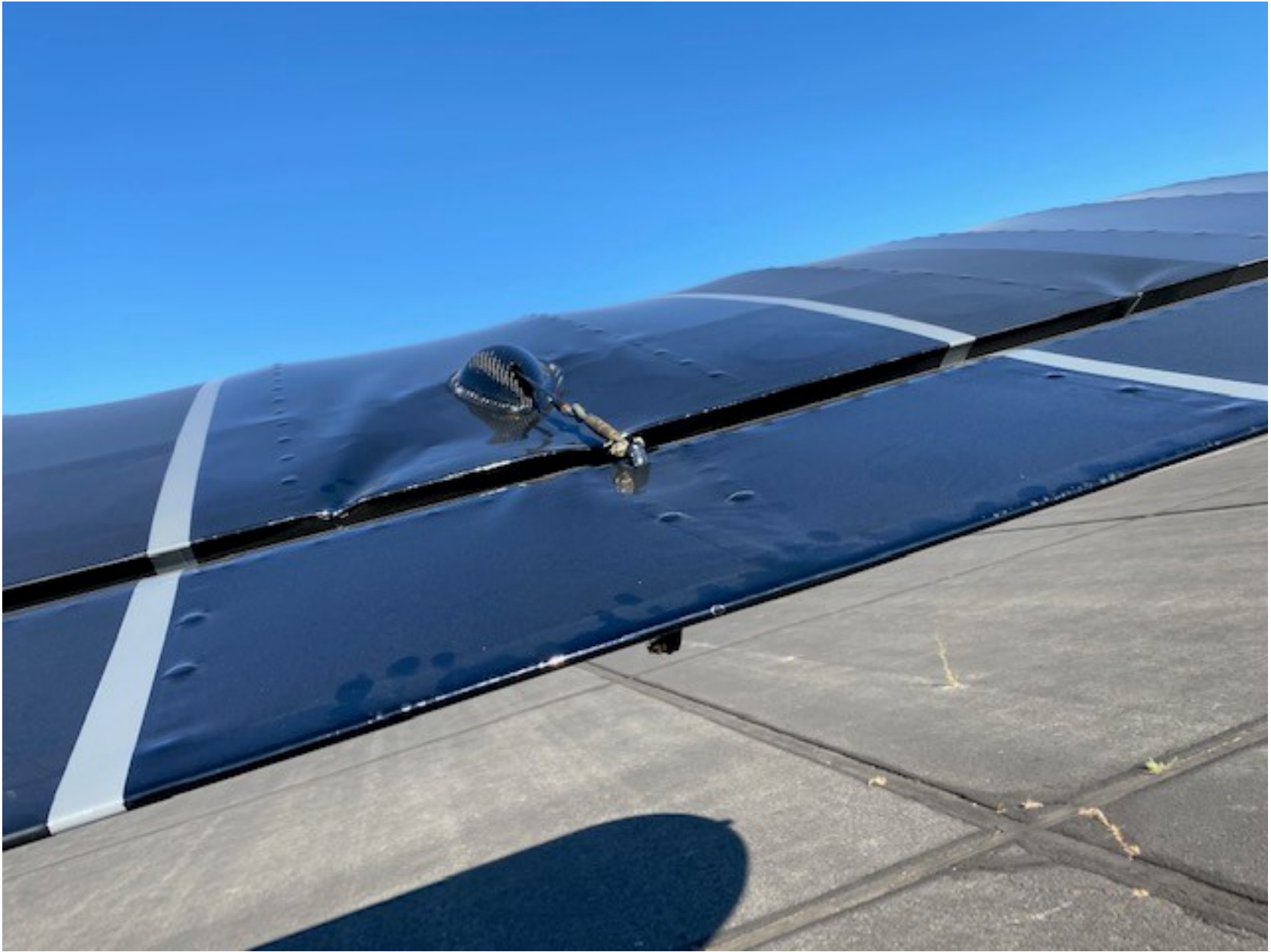
Photo 1 – Damage to the right wing. Photo courtesy of the pilot.
