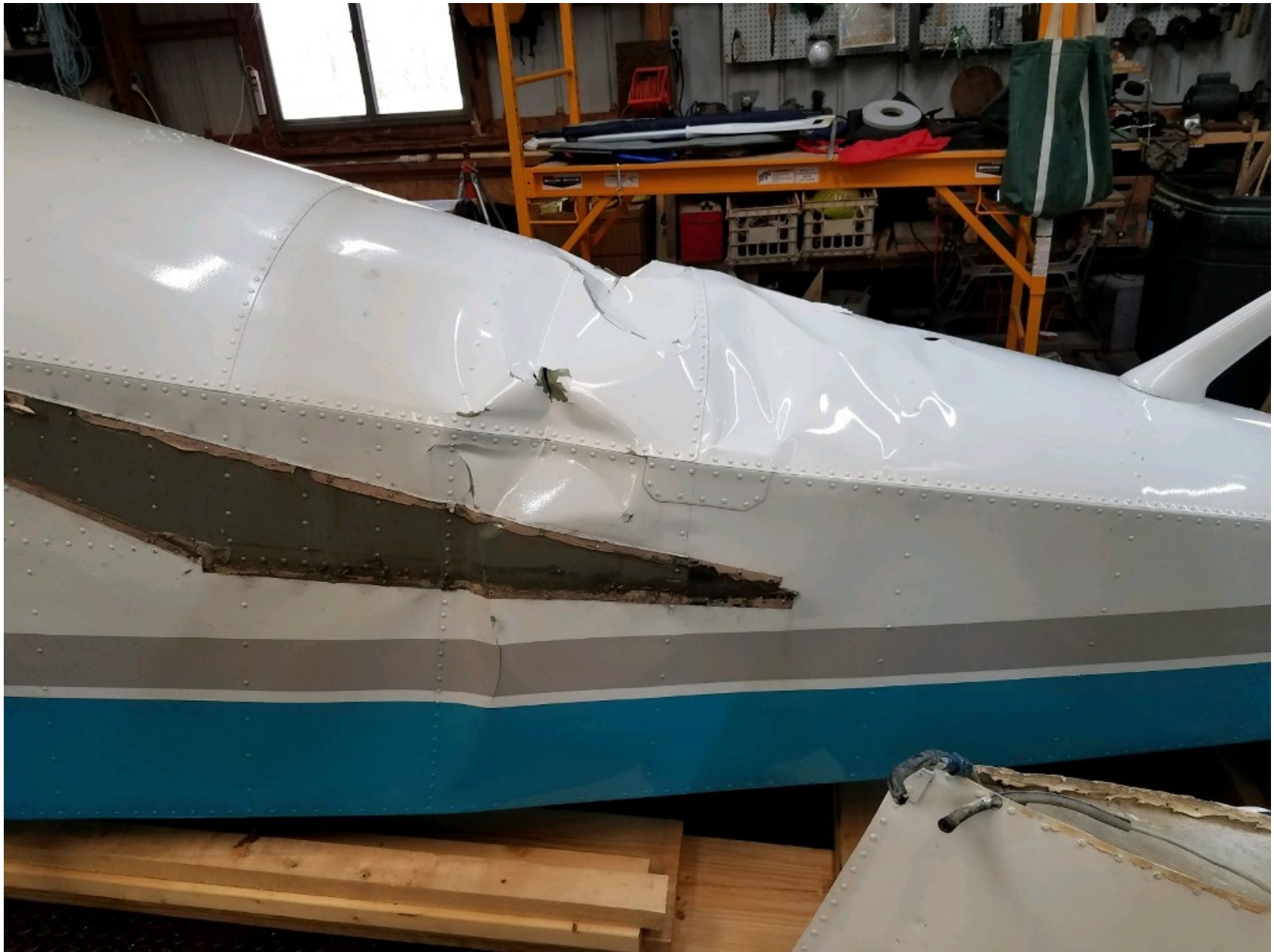
Photo 1 – Fuselage Damage (Owner's Photo)
