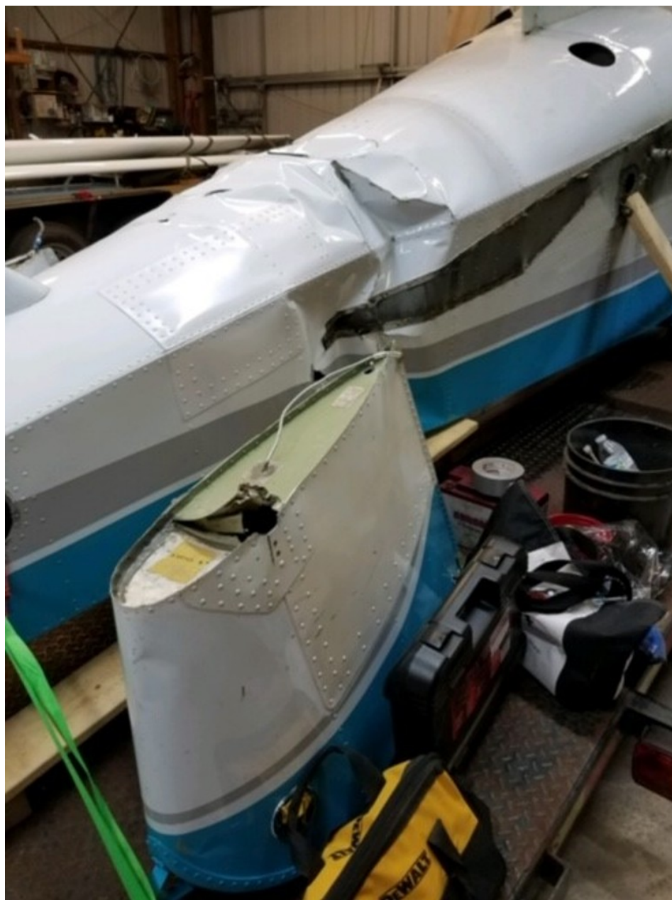
Photo 2 - Fuselage Damage (Owner's Photo)
