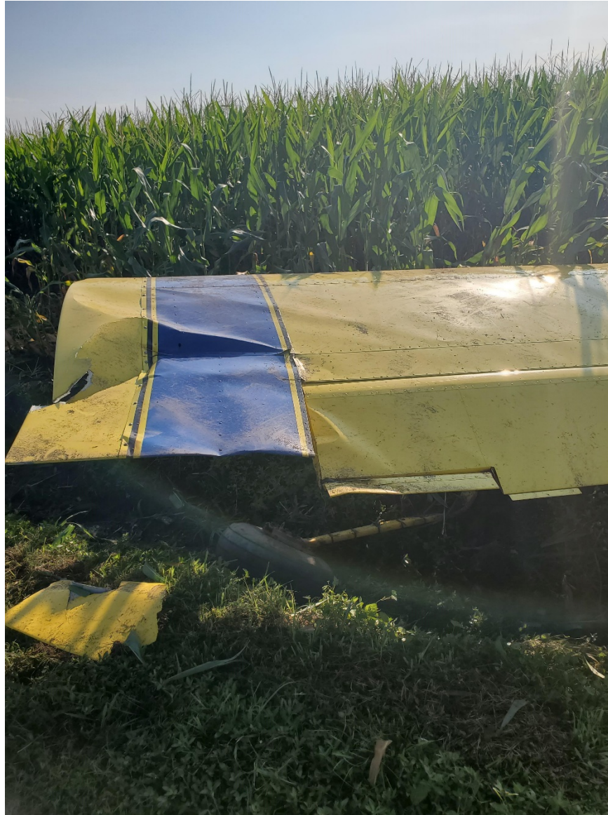
Photo 2 - Damage overview of outer left wing area (Photo Courtesy of FAA)
