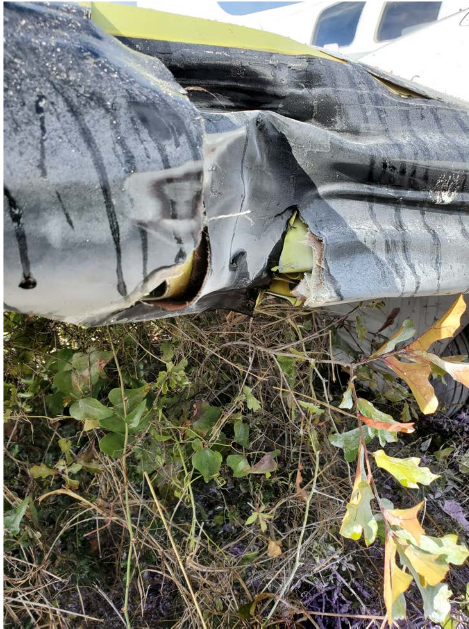
Photo 4 - Leading Edge of Right Wing – Courtesy of FAA
