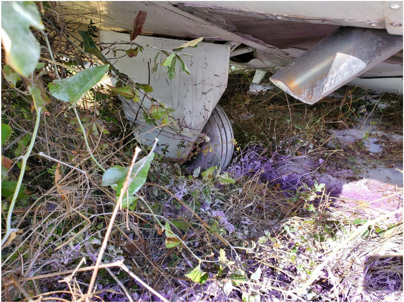
Photo 5 – Right Main Landing Gear – Courtesy of FAA
