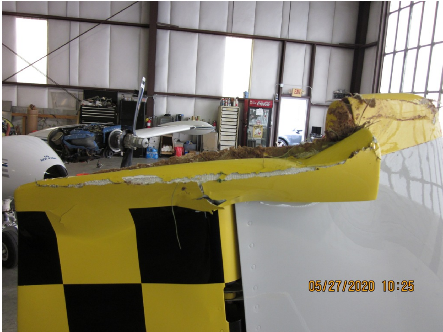
Photo 3 – Vertical Stabilizer Damage (Photo Courtesy of FAA)
