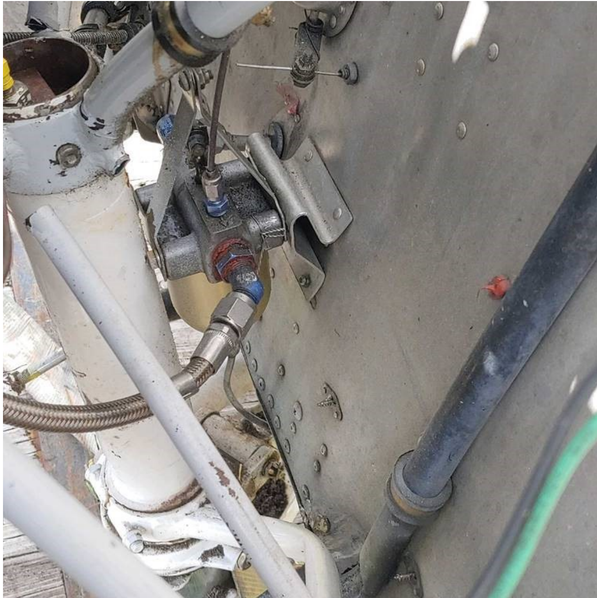
Photo 2 – View of substantially damaged engine mount (Photo Courtesy of FAA)
