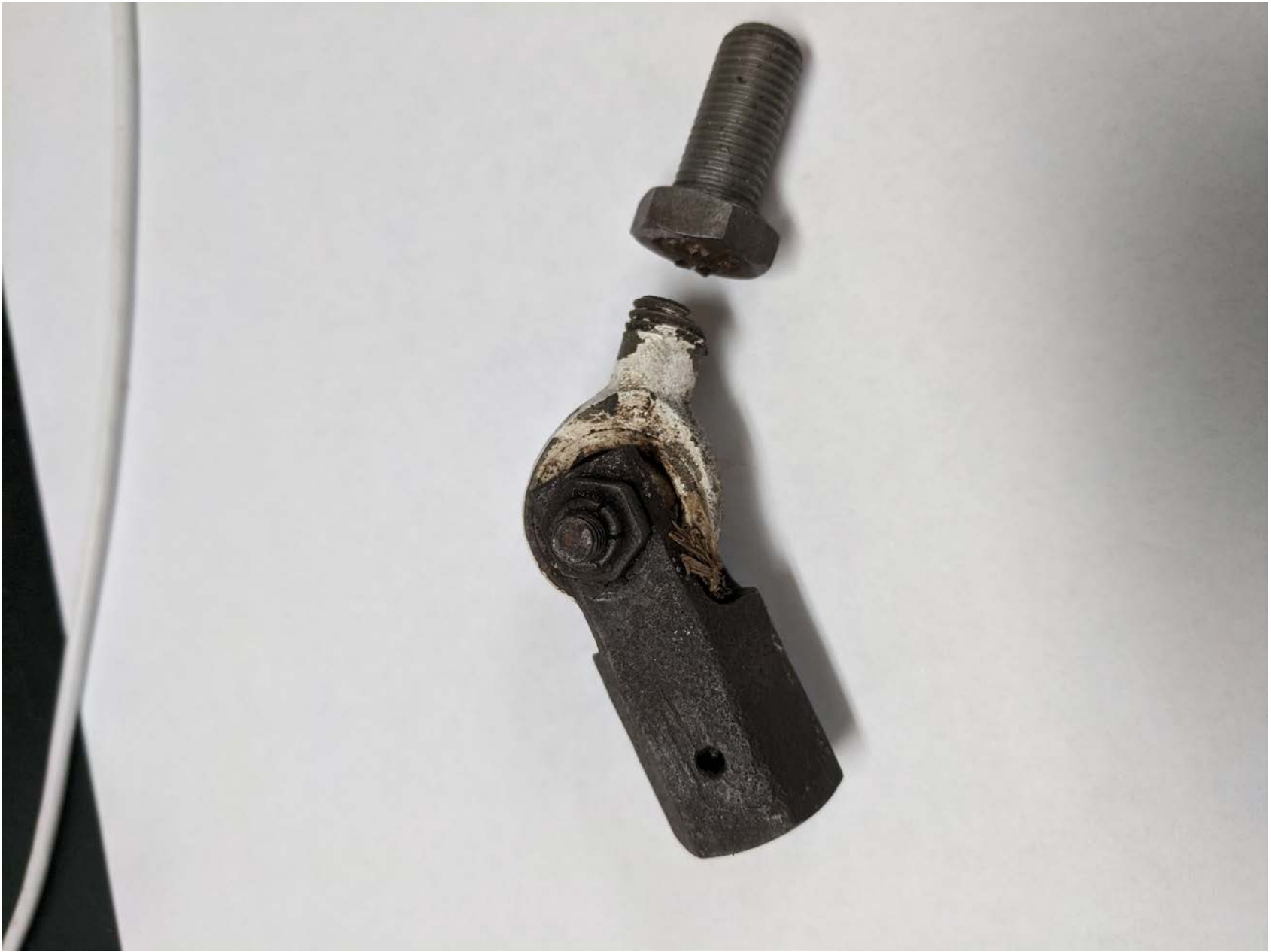
Photo 3 – View of failed nose steering rod end
