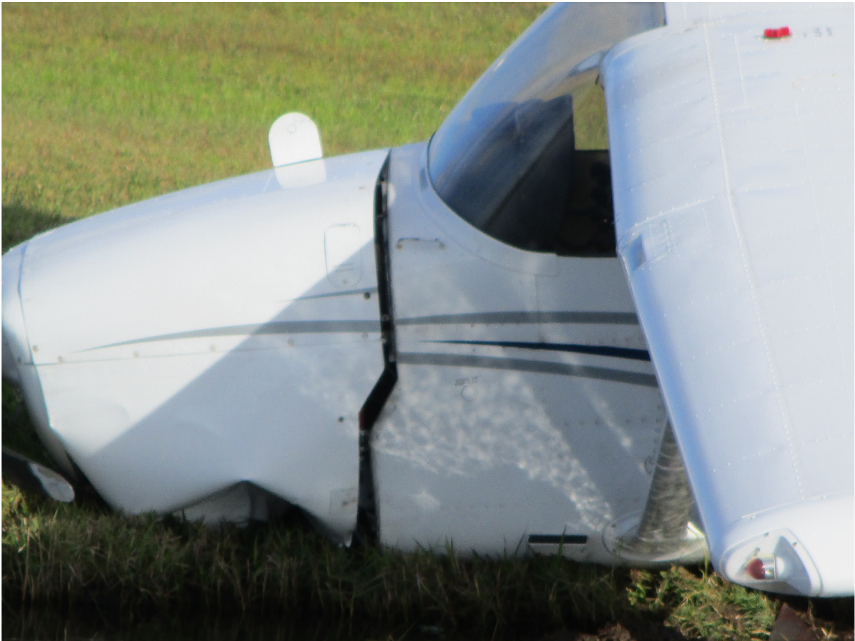
Photo 1 – View of nose of airplane on right side showing buckling of fuselage
