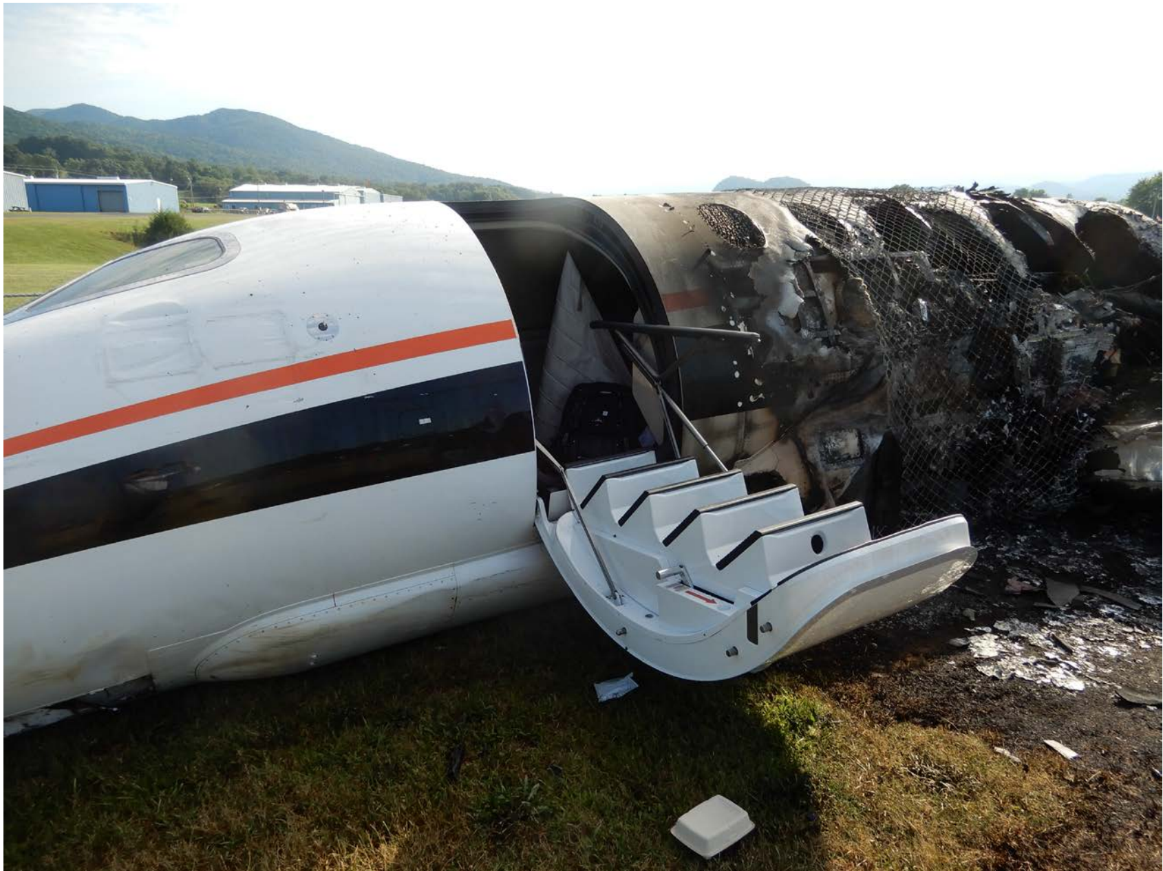
Photo 9 – Cabin Entry Door (NTSB Photo)
