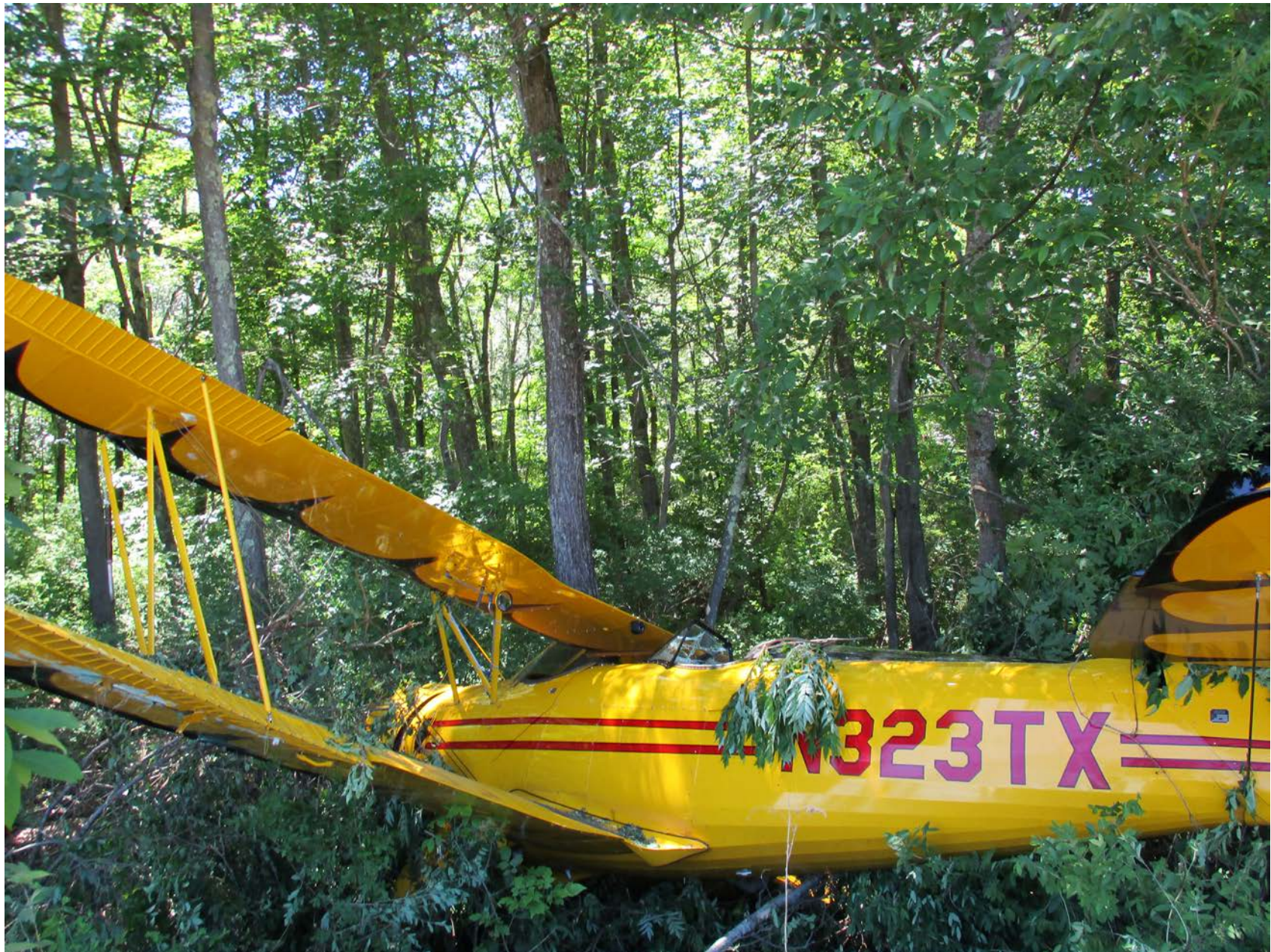
Photo 1 – View of airplane in heavy brush, upper wing fuselage buckled
