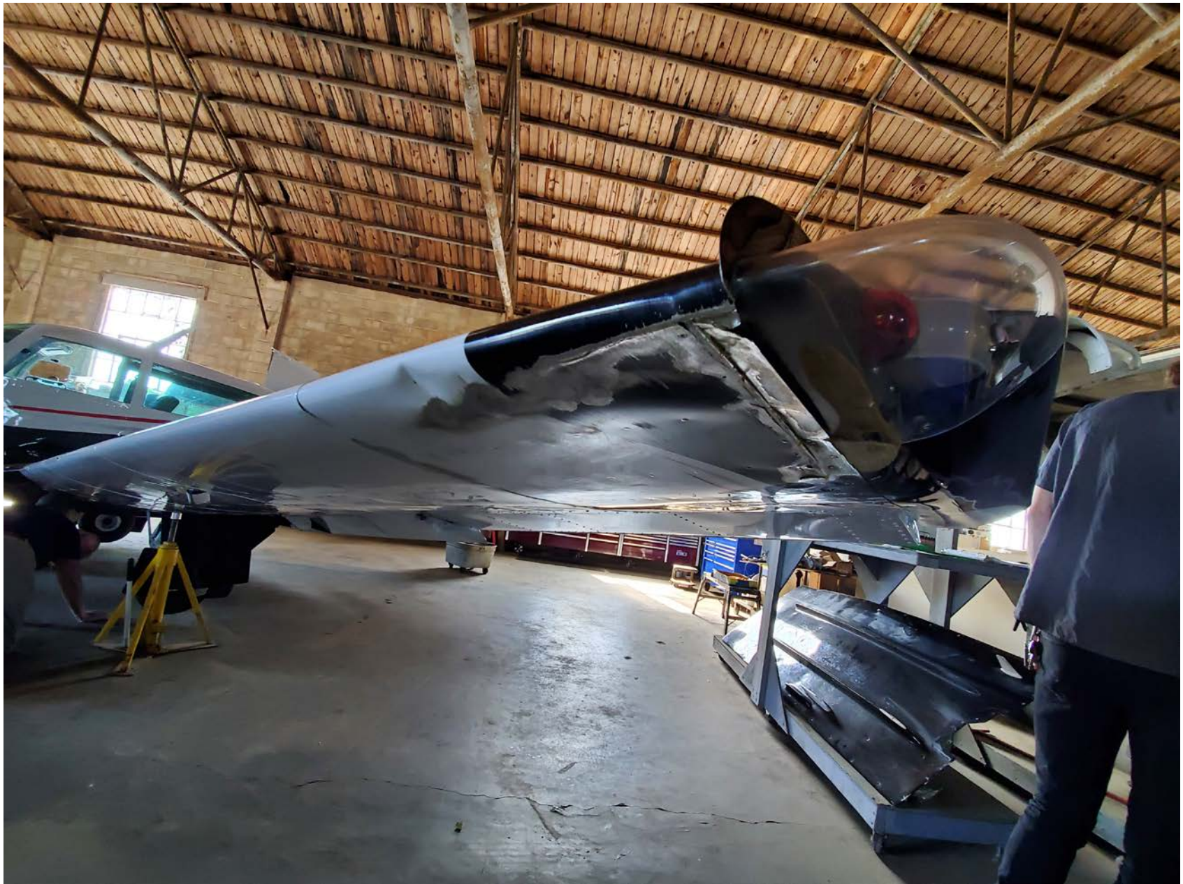
Photo 4 – View of left wing showing spar damage
