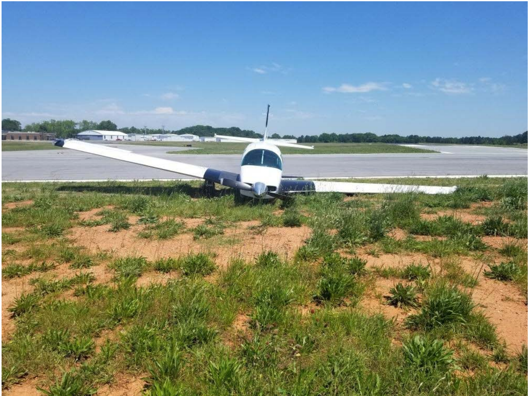
Photo 1 – View of front of airplane with left main landing gear collapsed
