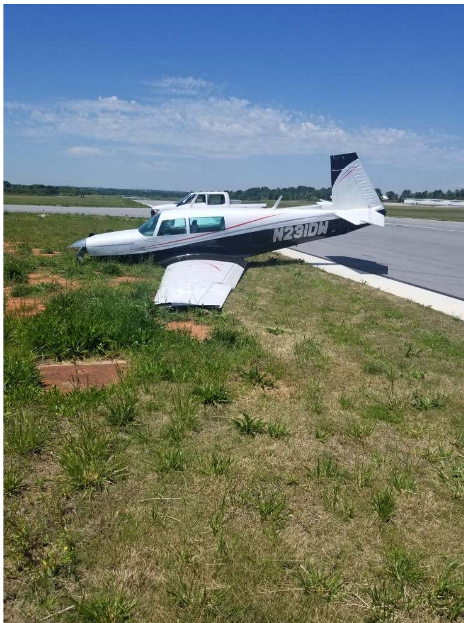
Photo 3 – View of left side of airplane showing left main collapsed gear
