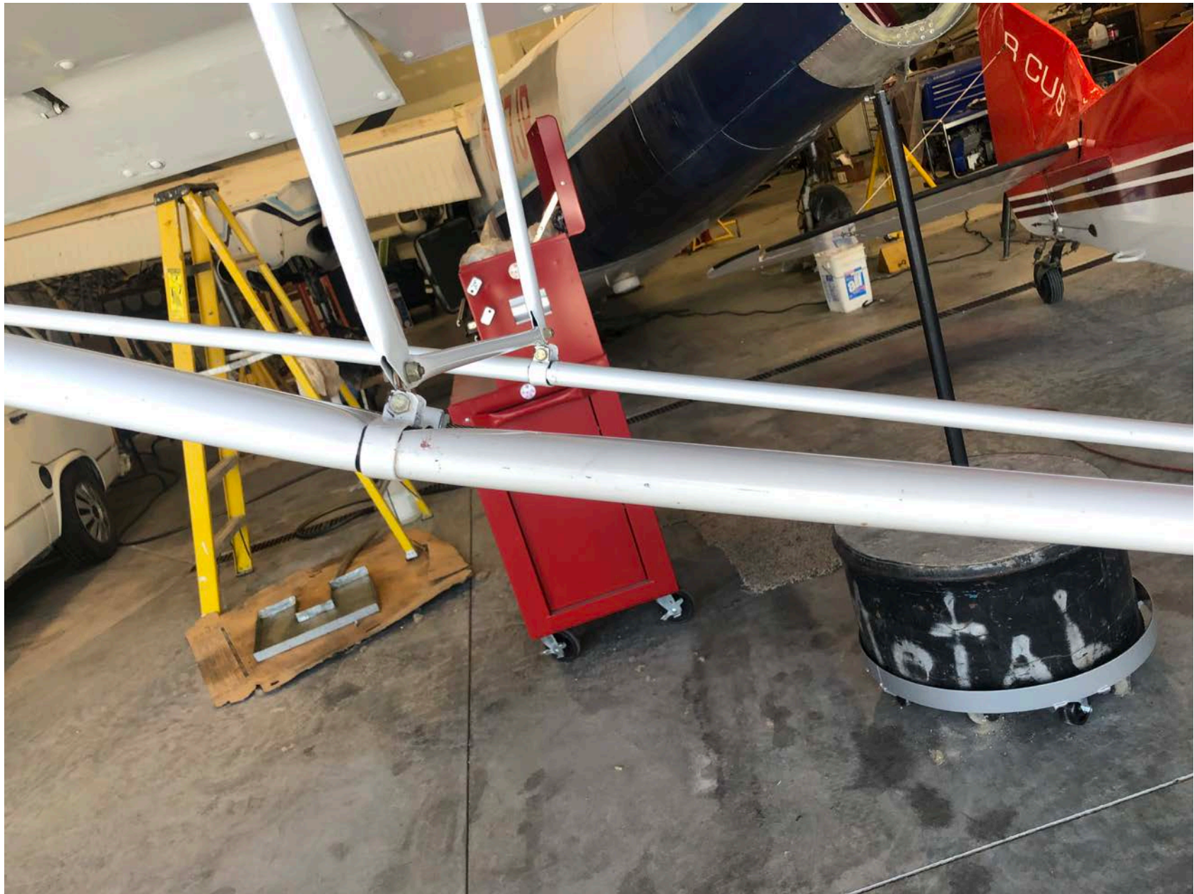
Photo 3 - Photo of the damaged right lift strut. Photo courtesy of McLarens Insurance Company.
