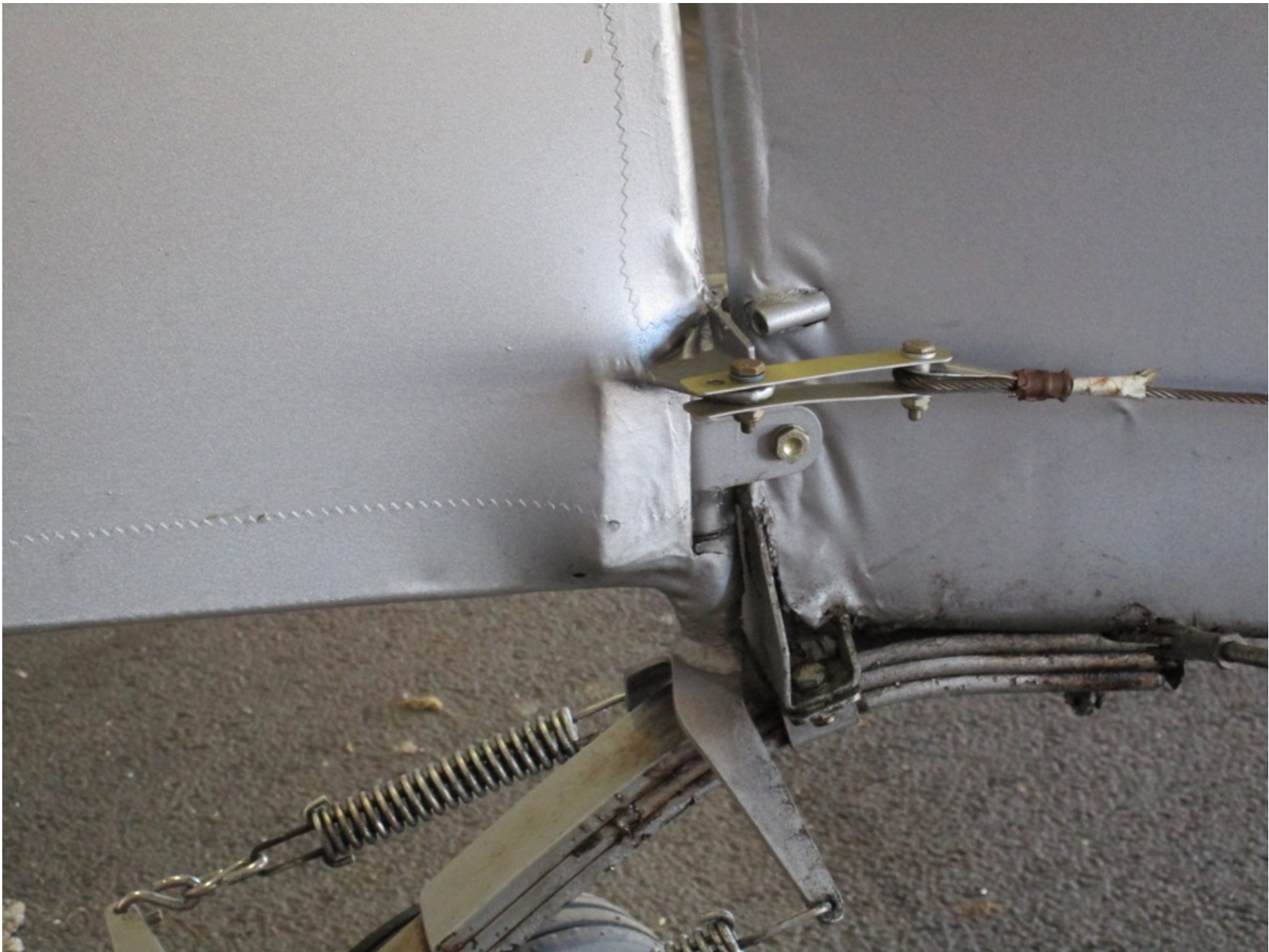
Photo 3 – Tailwheel And Airframe Damage (Photo Courtesy of FAA)
