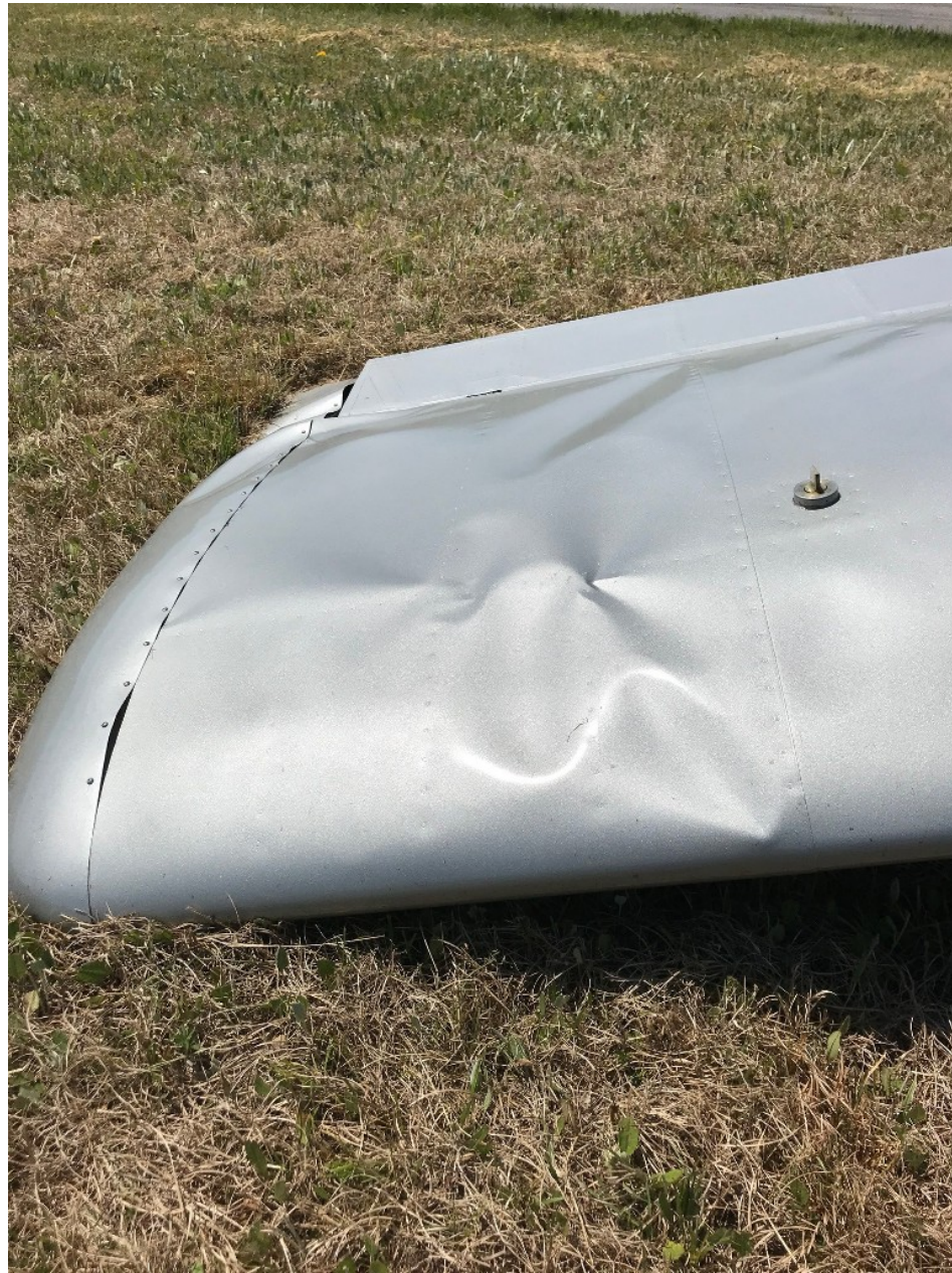
Photo 2 – Right Wing Damage (Photo Courtesy of Airport Manager)
