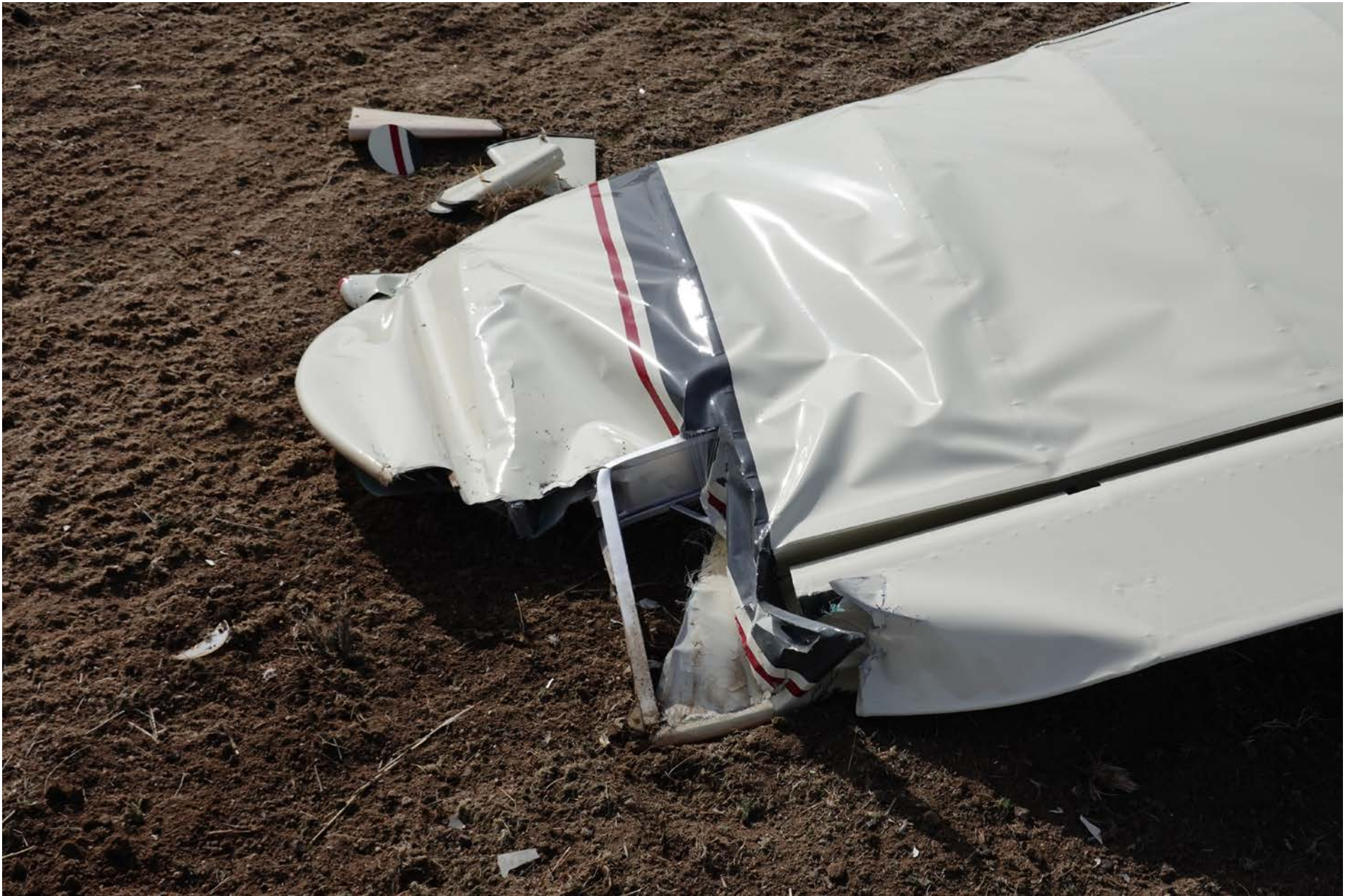
Photo 2 – Damage to left wing
