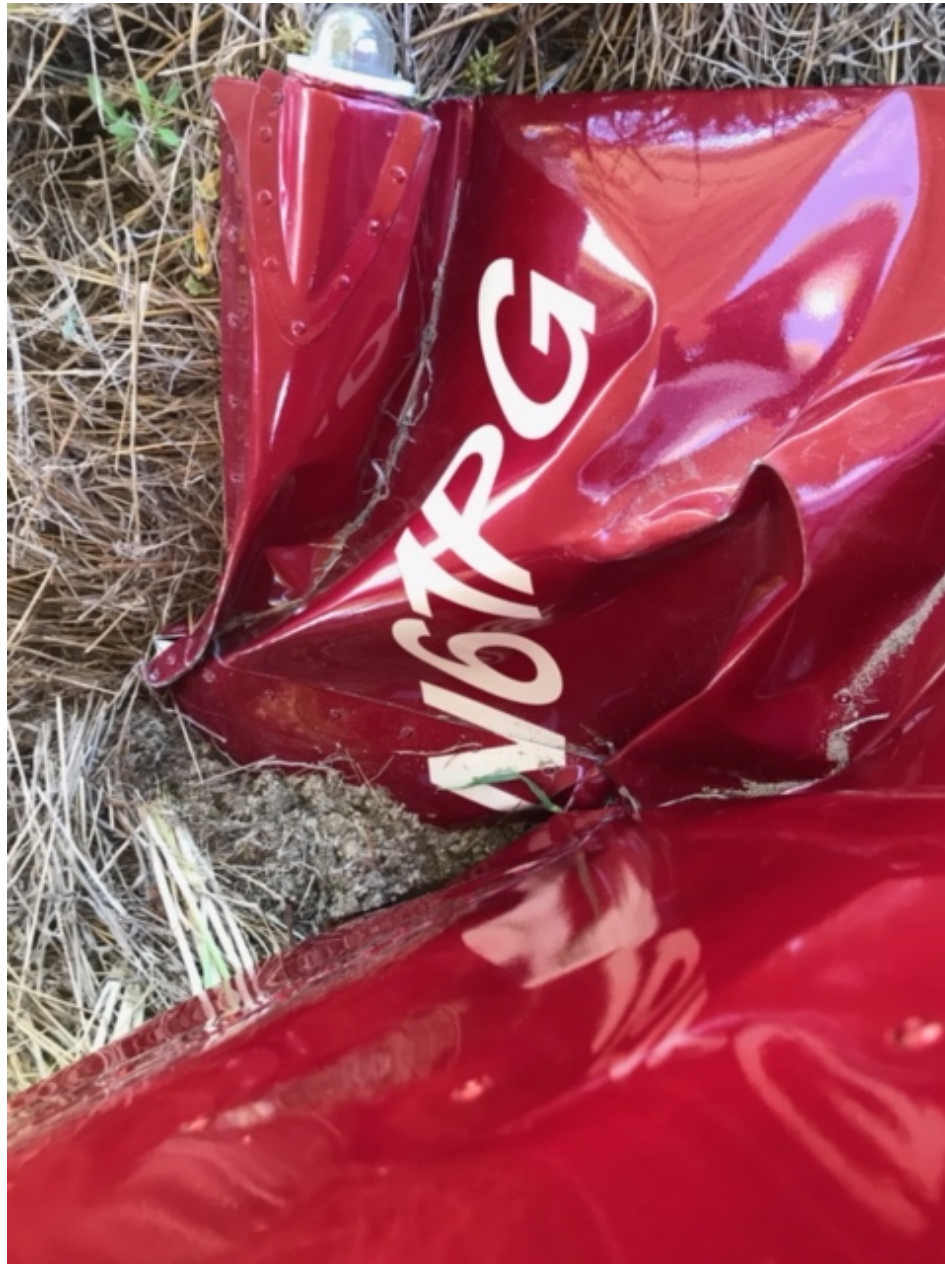
Photo 3 – View of Substantially Damaged Rudder (Photo Courtesy of FAA)
