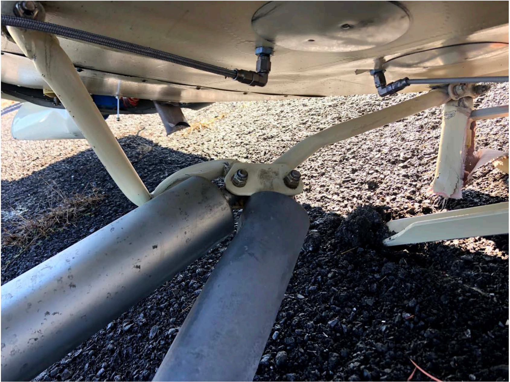
Photo 5 – View of Fractured Right Main Landing Gear Leg (FAA)
