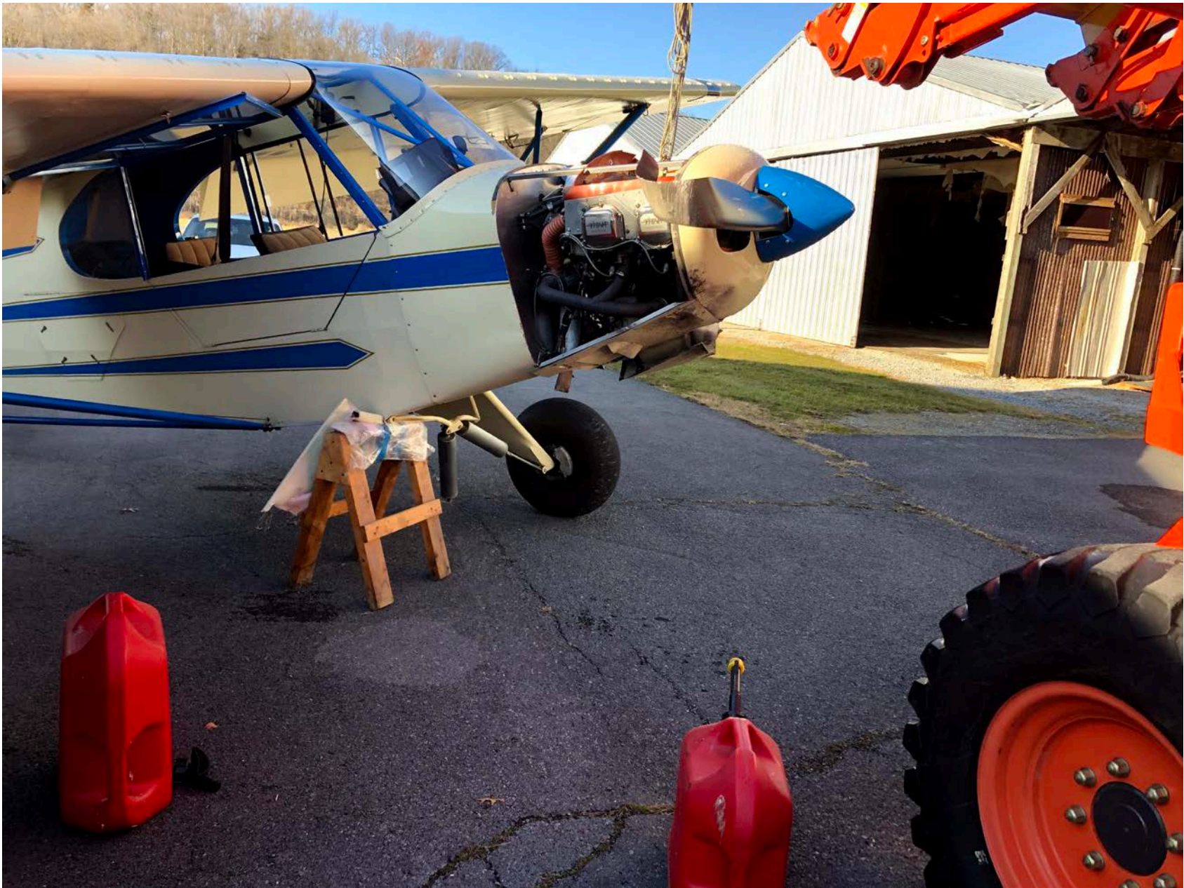
Photo 4 – View of Landing Gear Dampeners and Deformed Dampener Mounts after Recovery (FAA)
