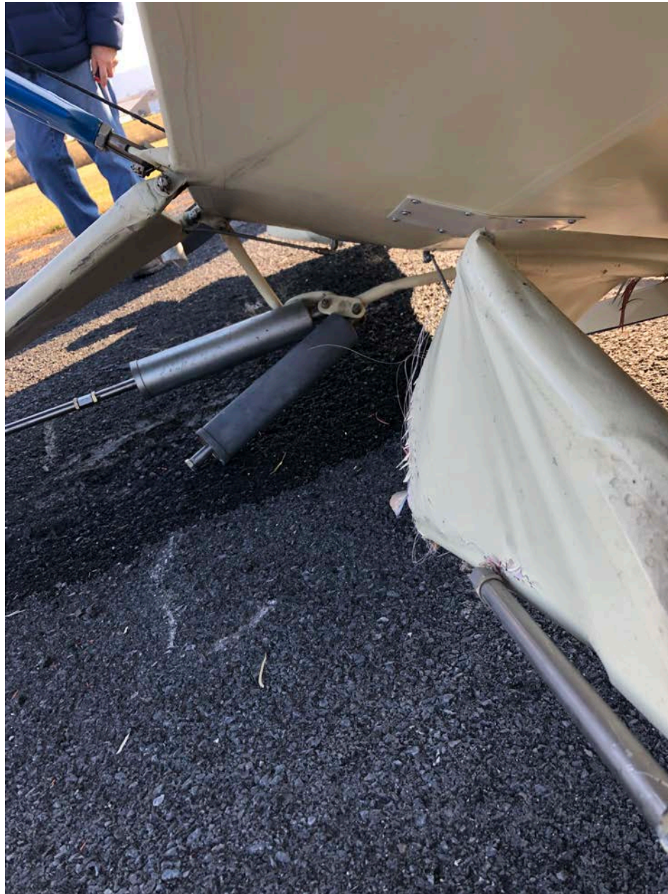
Photo 3 – View of Both Dampeners at the Accident Site (FAA)
