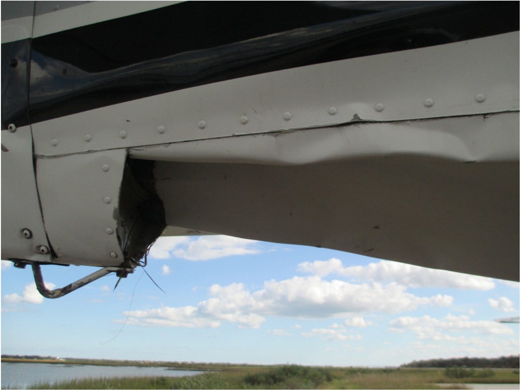
Photo 4 – Empennage Damage (Photo Courtesy of FAA)
