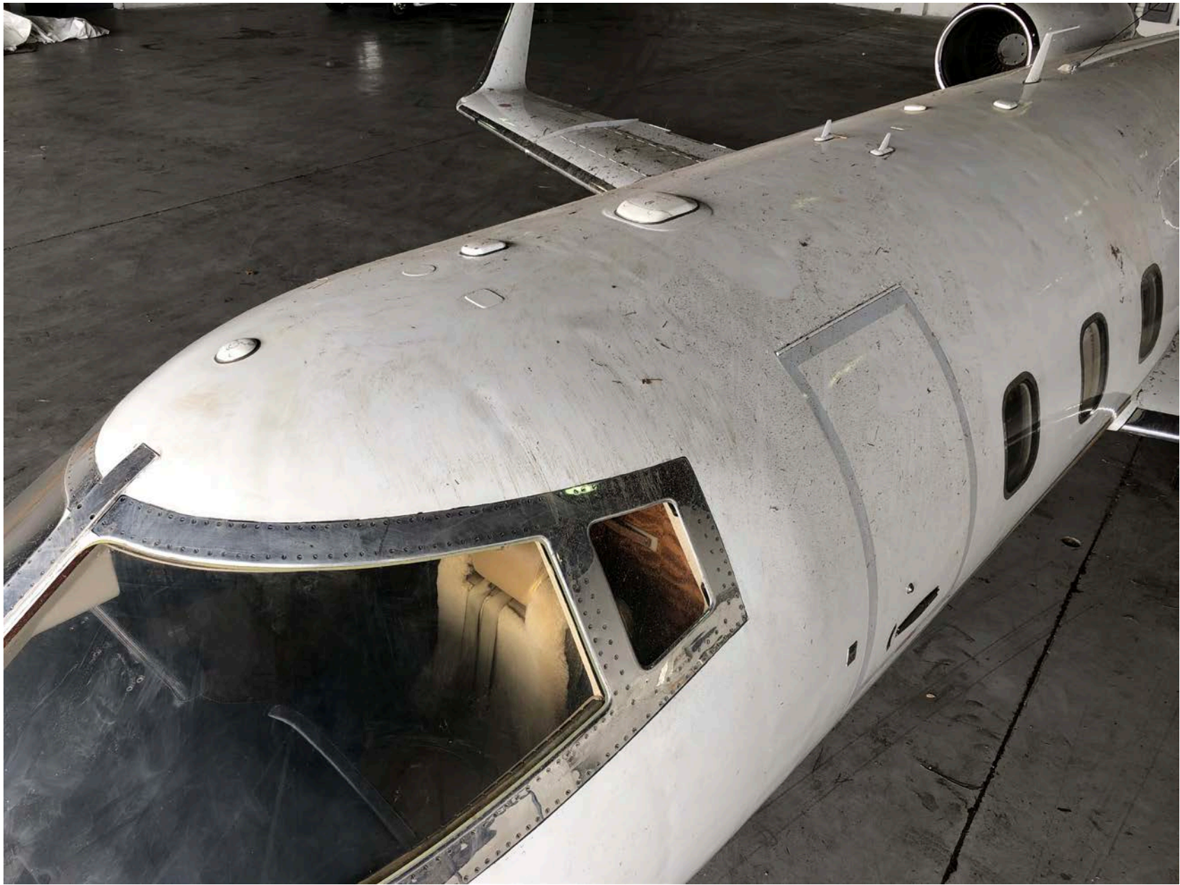
Photo 4 - View of top of airplane showing buckling on the top of the fuselage
