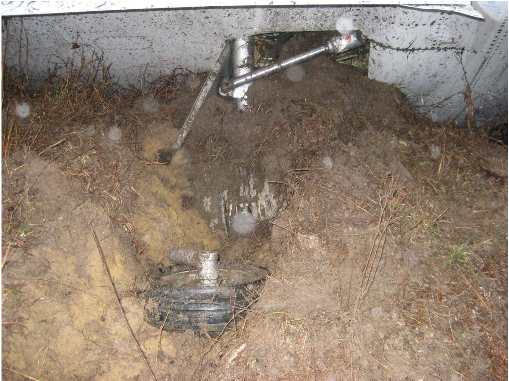
Photo 2 – View of broken nose gear
