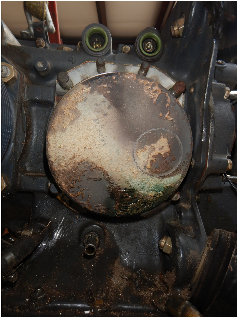
Photo 10 – Cylinder No. 4 Piston Face
