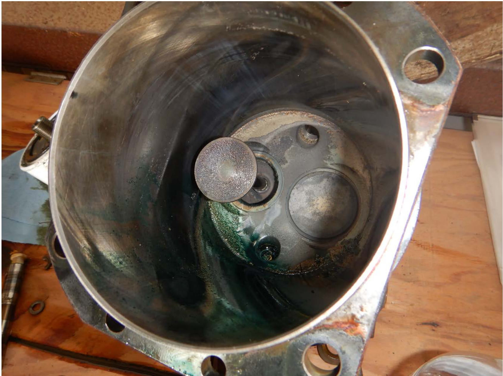
Photo 11 – Cylinder No. 4 Exhaust and Intake Valves
