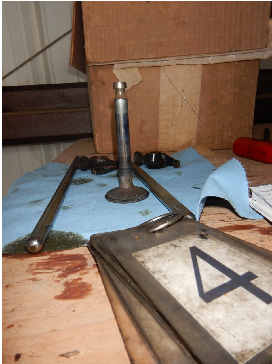
Photo 12 – Cylinder No. 4 Exhaust Valve Stem
