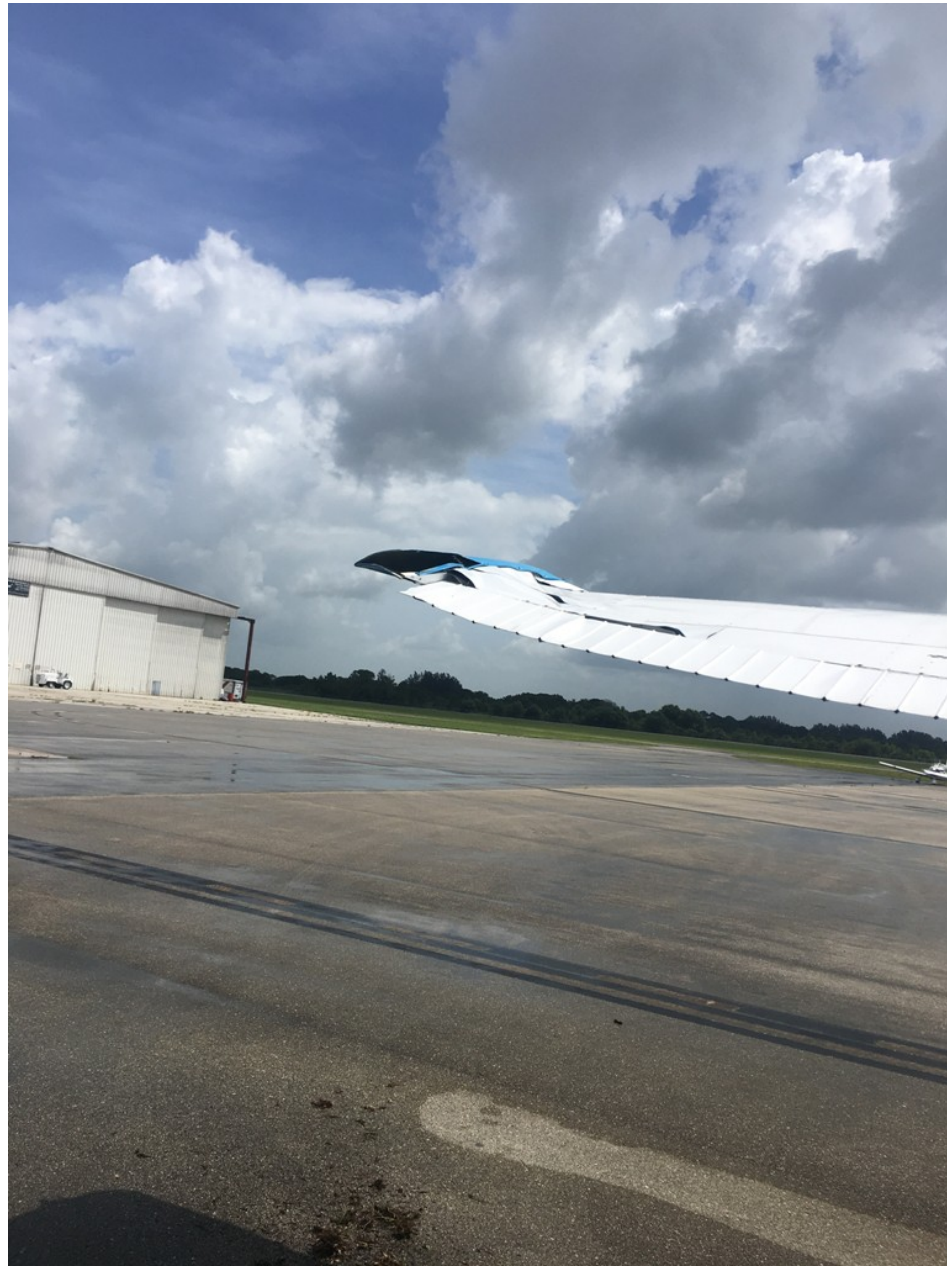
Photo 2 – Left Wing Damage (Photo Courtesy of Pilot)
