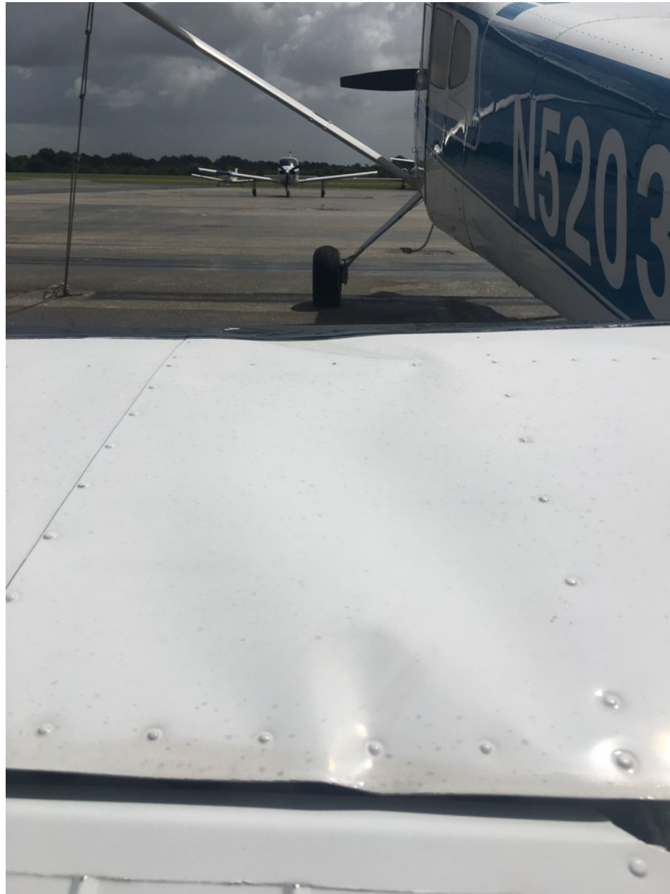
Photo 3 – Left Horizontal Stabilizer Damage (Photo Courtesy of Pilot)
