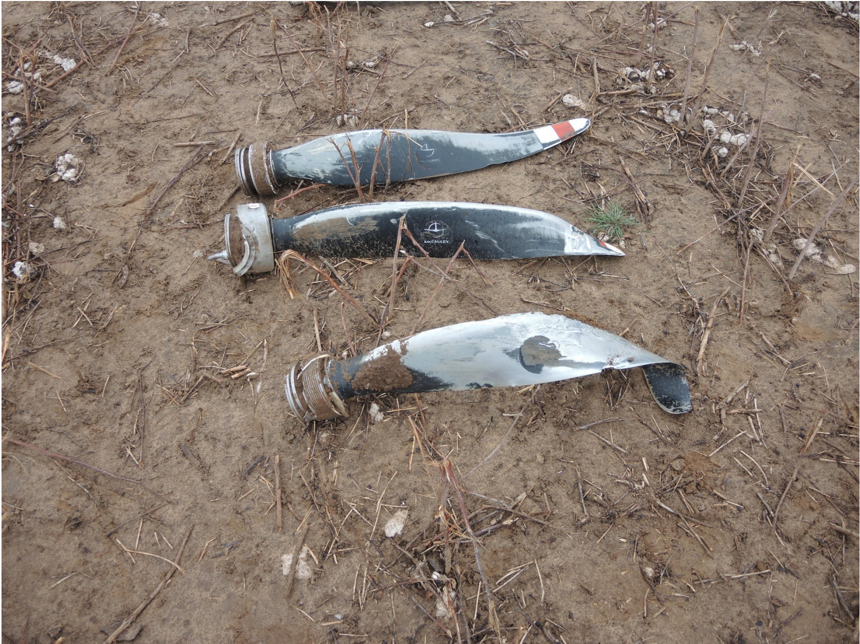
Photo 4 – View of the propellers, once placed together for photo at the accident site
