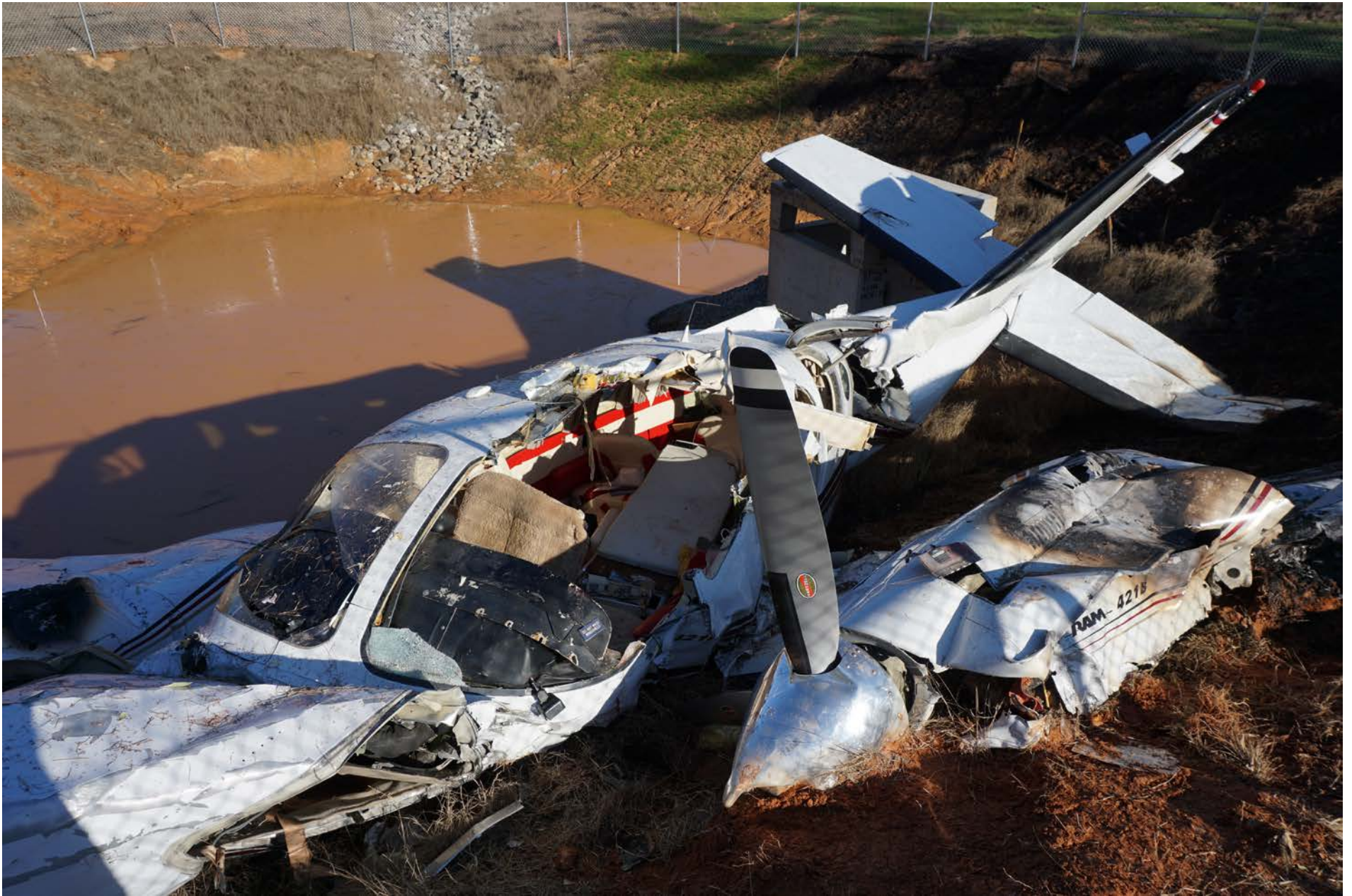
Photo 4 – Left side of airplane wreckage showing left engine and fuselage in retention pond bank.
