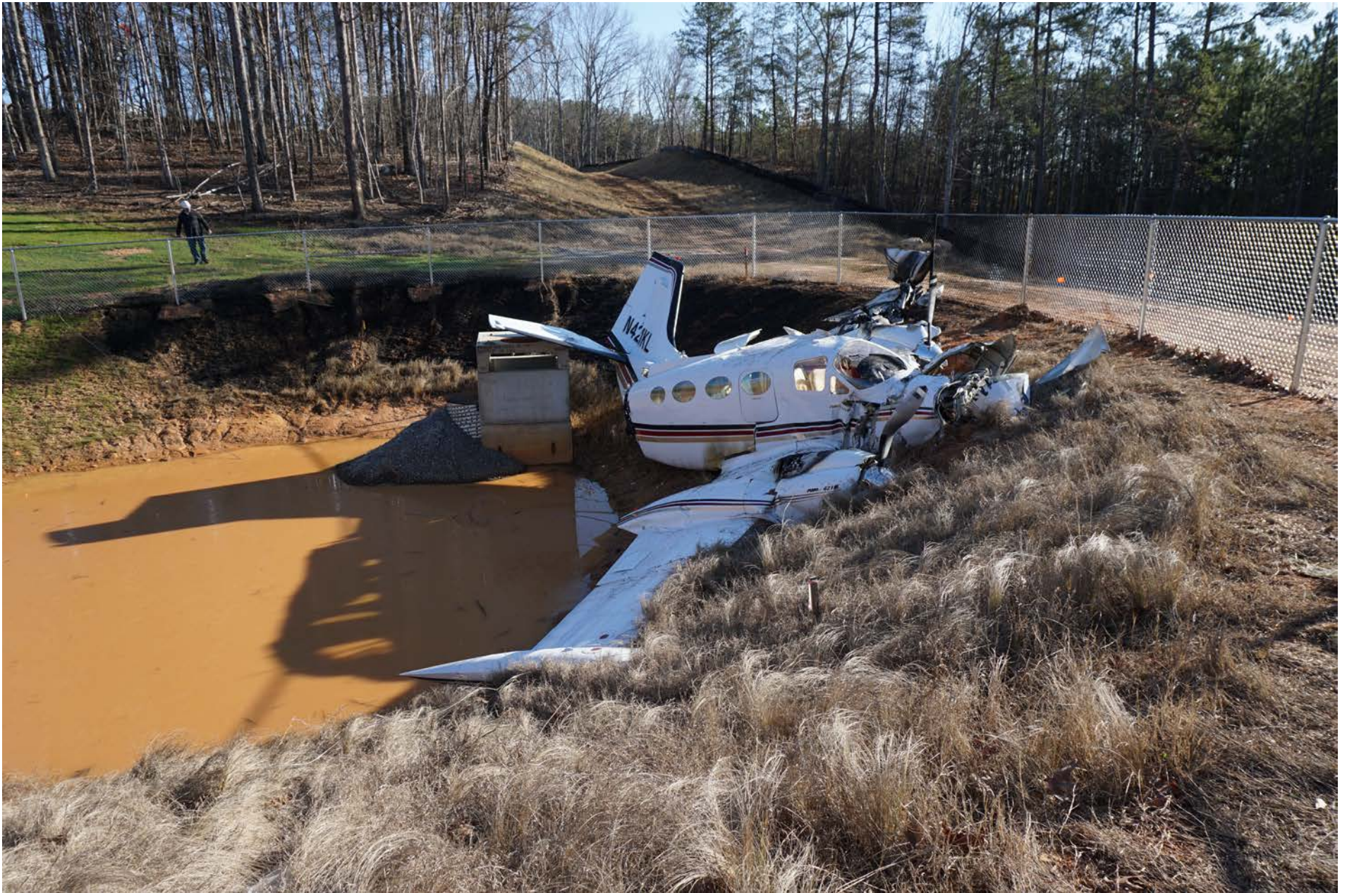
Photo 2 – View of right side of airplane wreckage showing right engine and fuselage on the bank of the retention pond.
