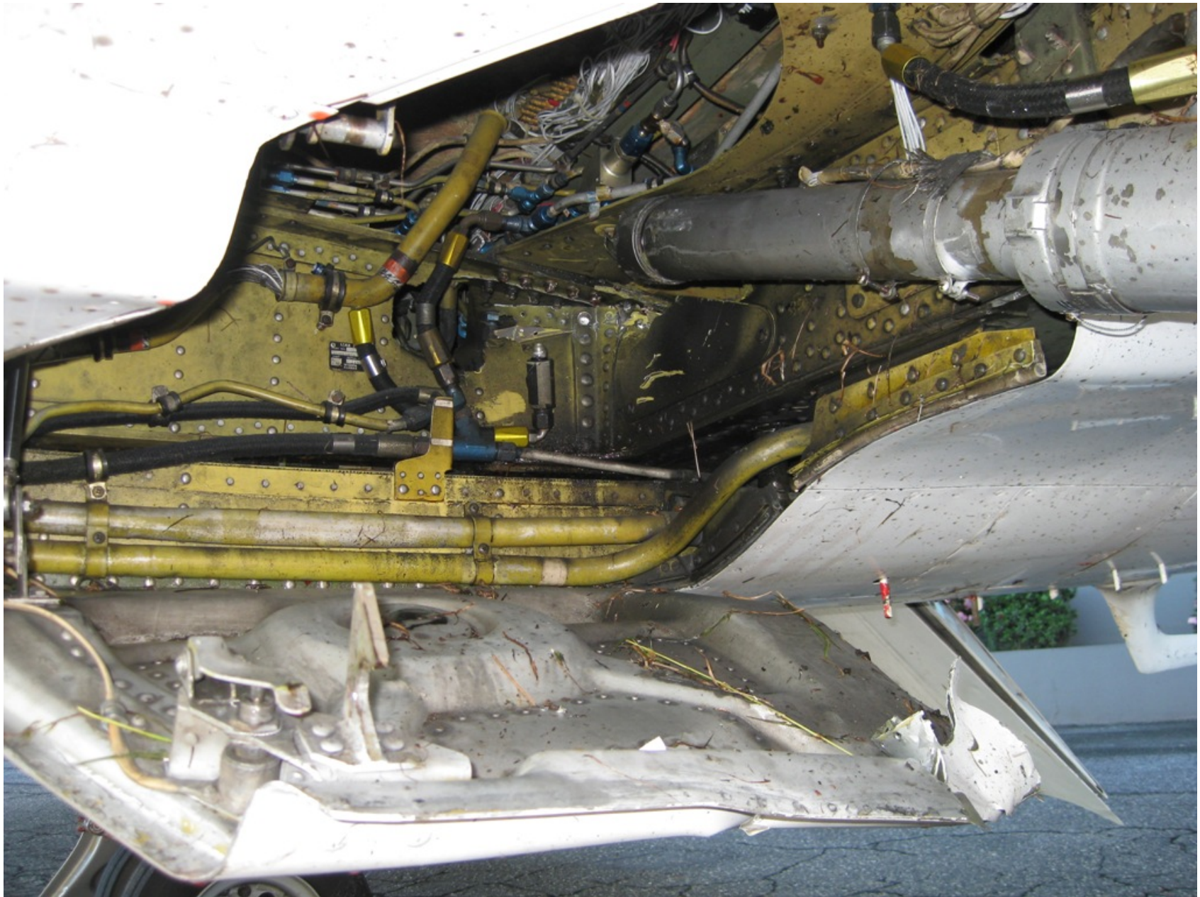
Photo 2 – Left Main Wheel Well Structural Damage (FAA Photo)
