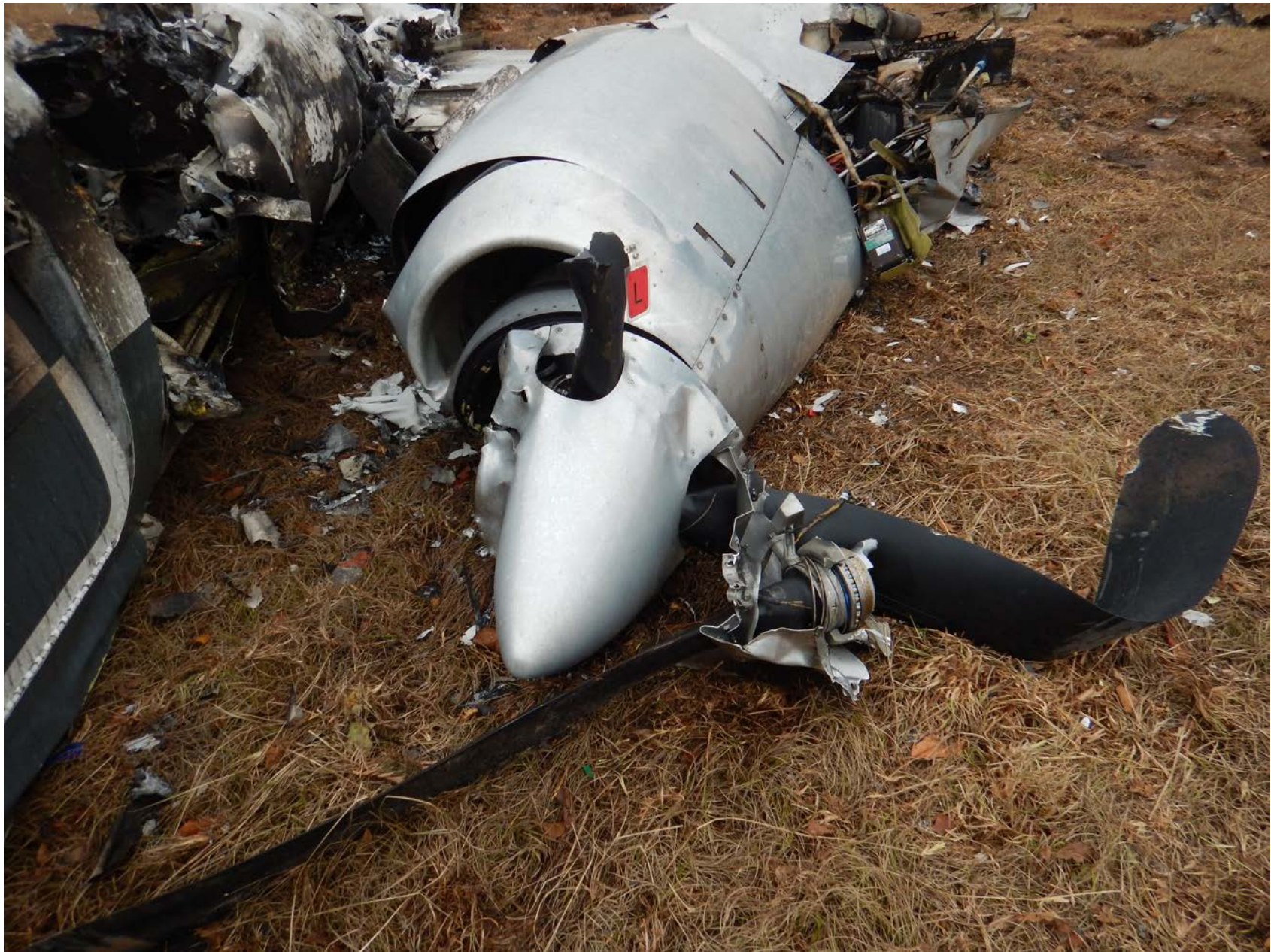
Photo 15 – View of damaged left engine
