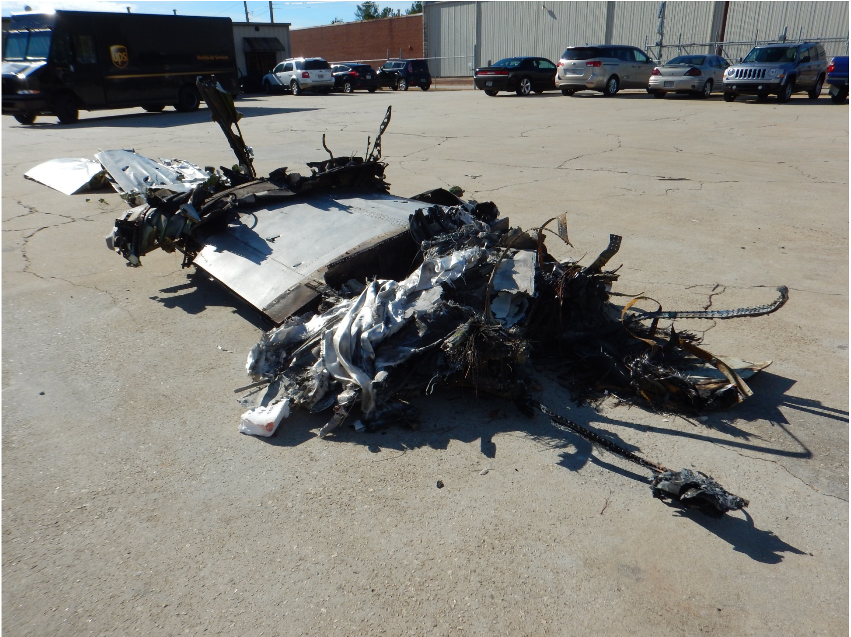
Photo 10 – View of left wing section damaged
