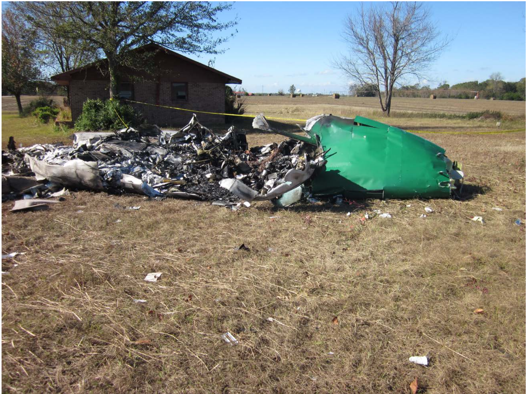
Photo 3 – Right side view of cockpit and nose fire damaged
