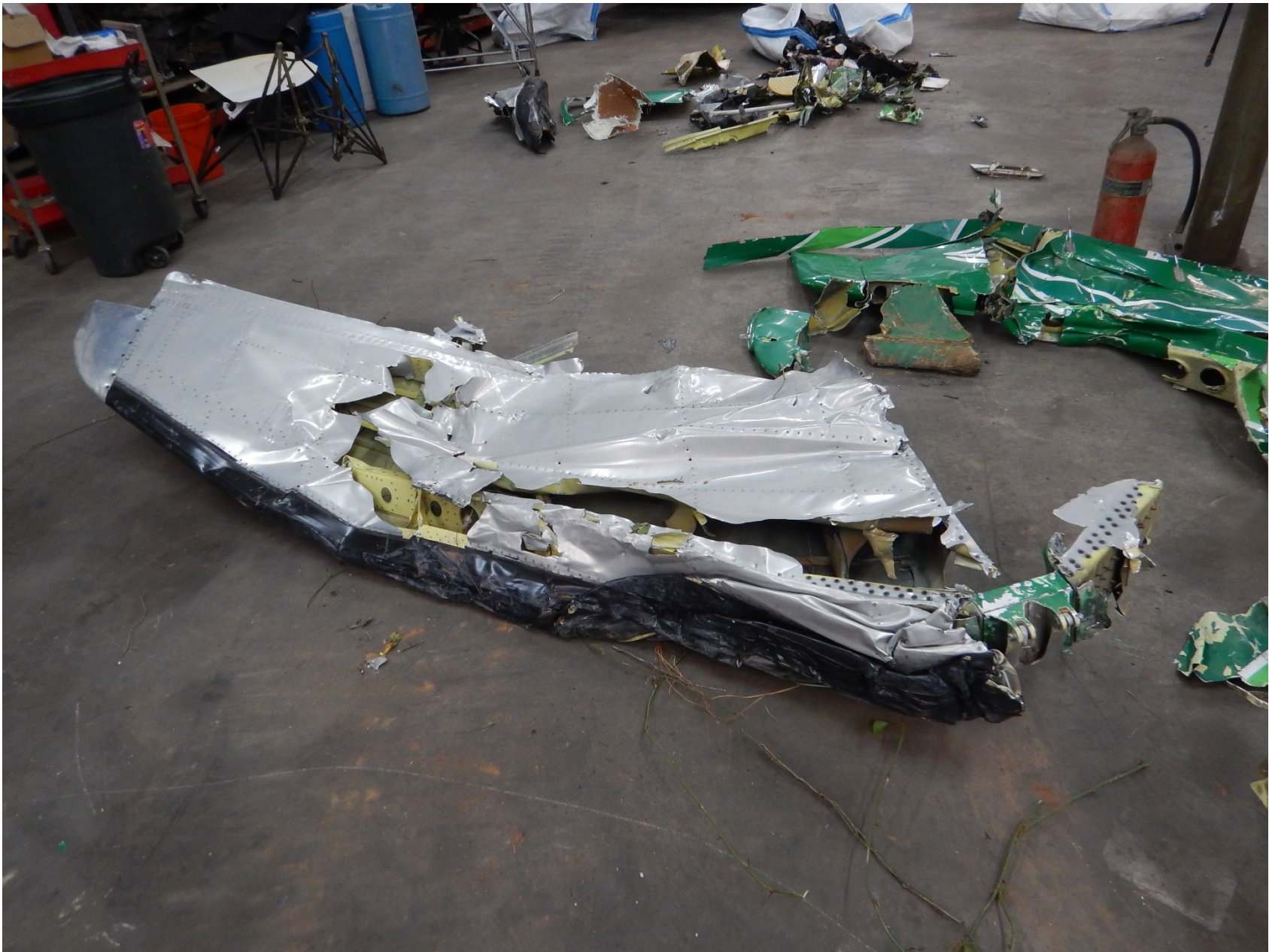
Photo 8 – View of a right side section of the horizontal stabilizer
