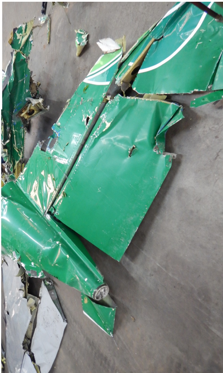
Photo 7 – View of a section of the rudder
