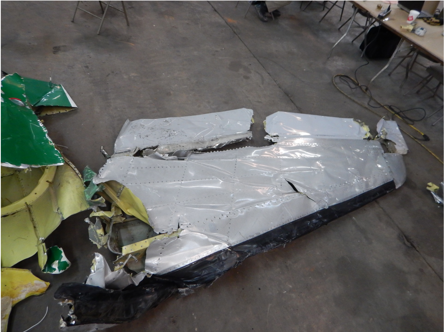
Photo 9 – View of a left side section of the horizontal stabilizer and damaged elevator sections
