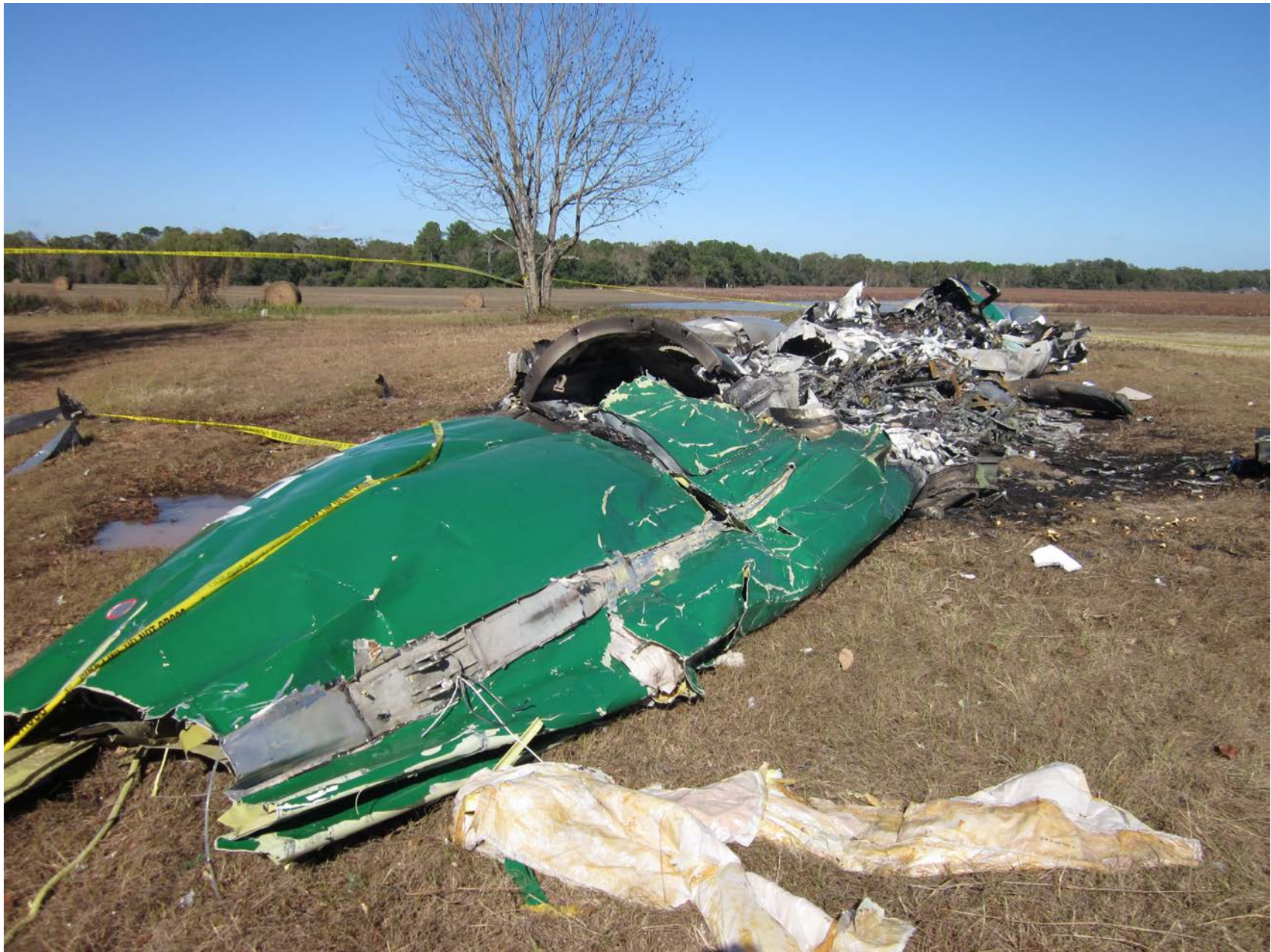
Photo 2 – View of aft section of fuselage showing crush damage
