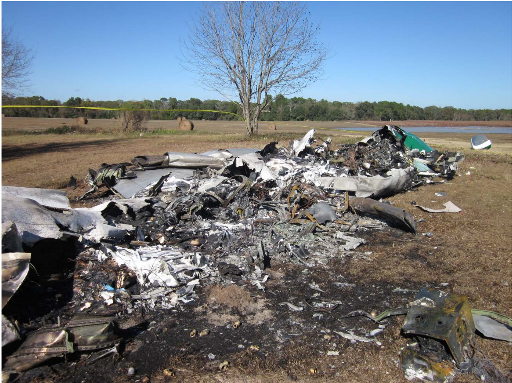
Photo 1 – View of main wreckage showing fire damaged fuselage
