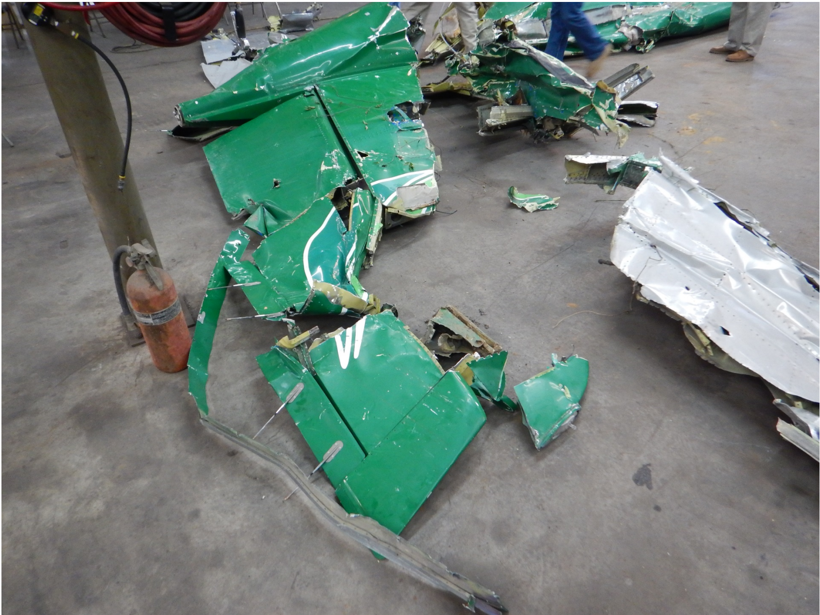
Photo 6 – View of a section of the vertical stabilizer and rudder attached to part of the tail section
