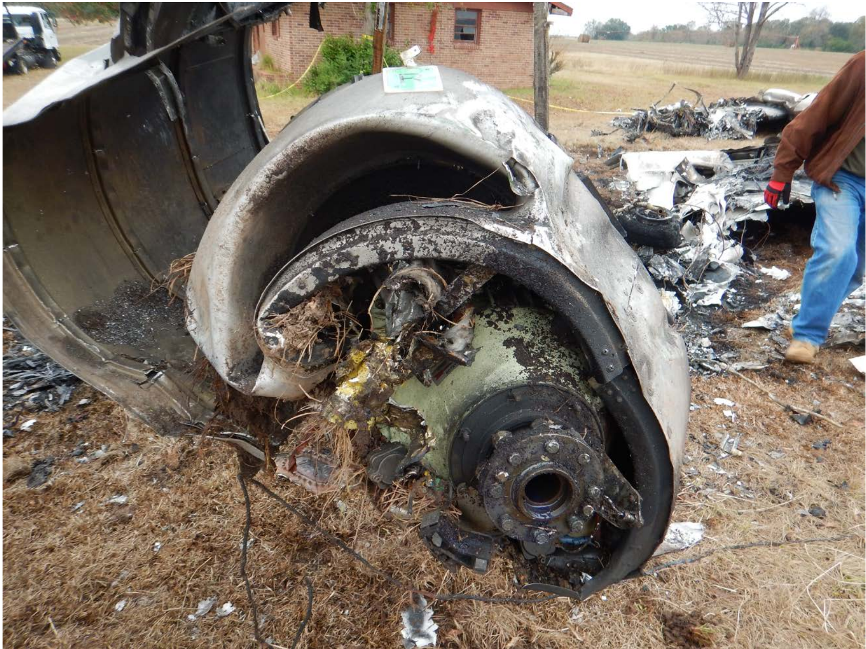
Photo 14 – View of damaged right engine
