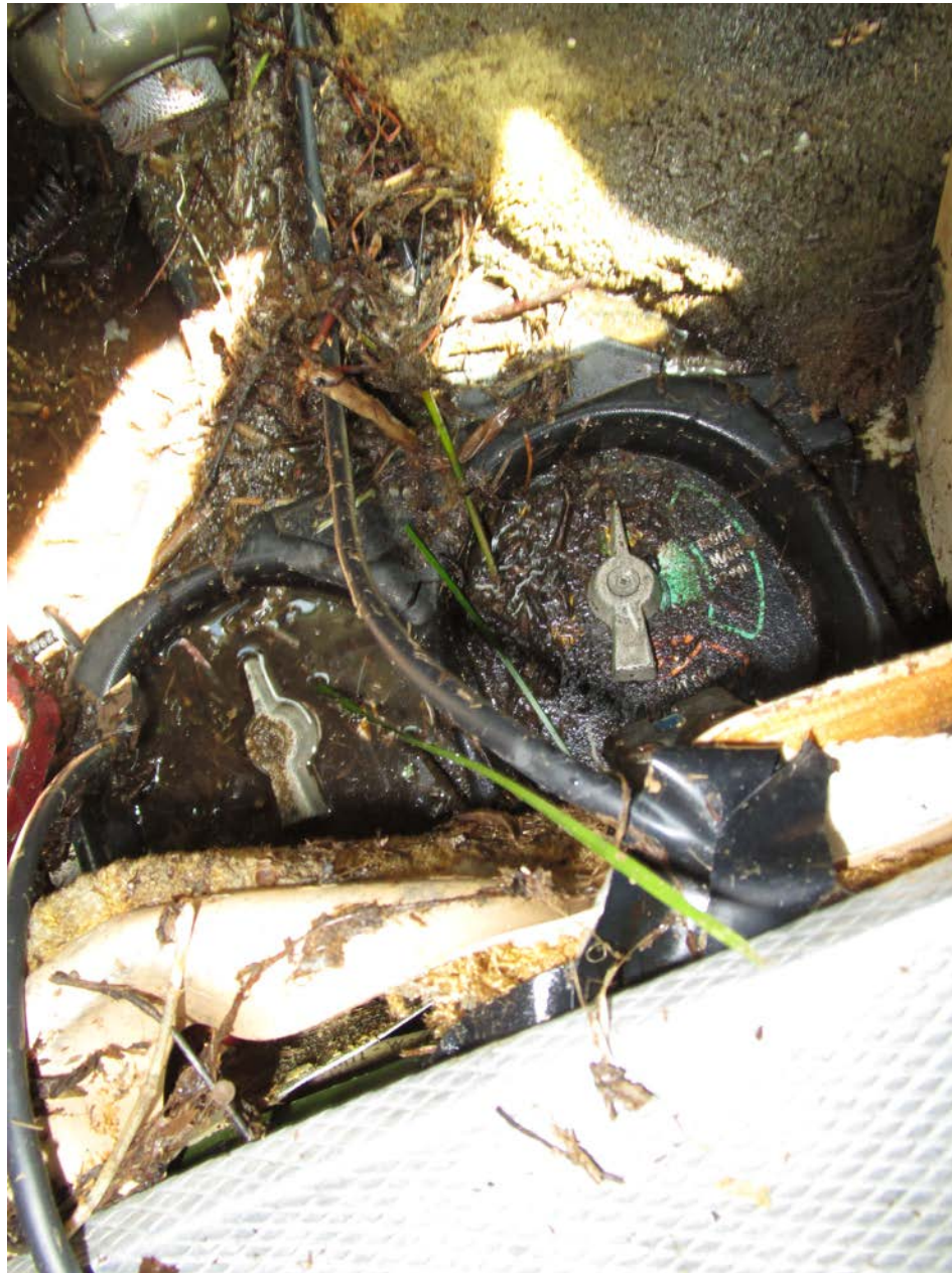
Photo 3 – View of Fuel Selectors as Found (FAA)
