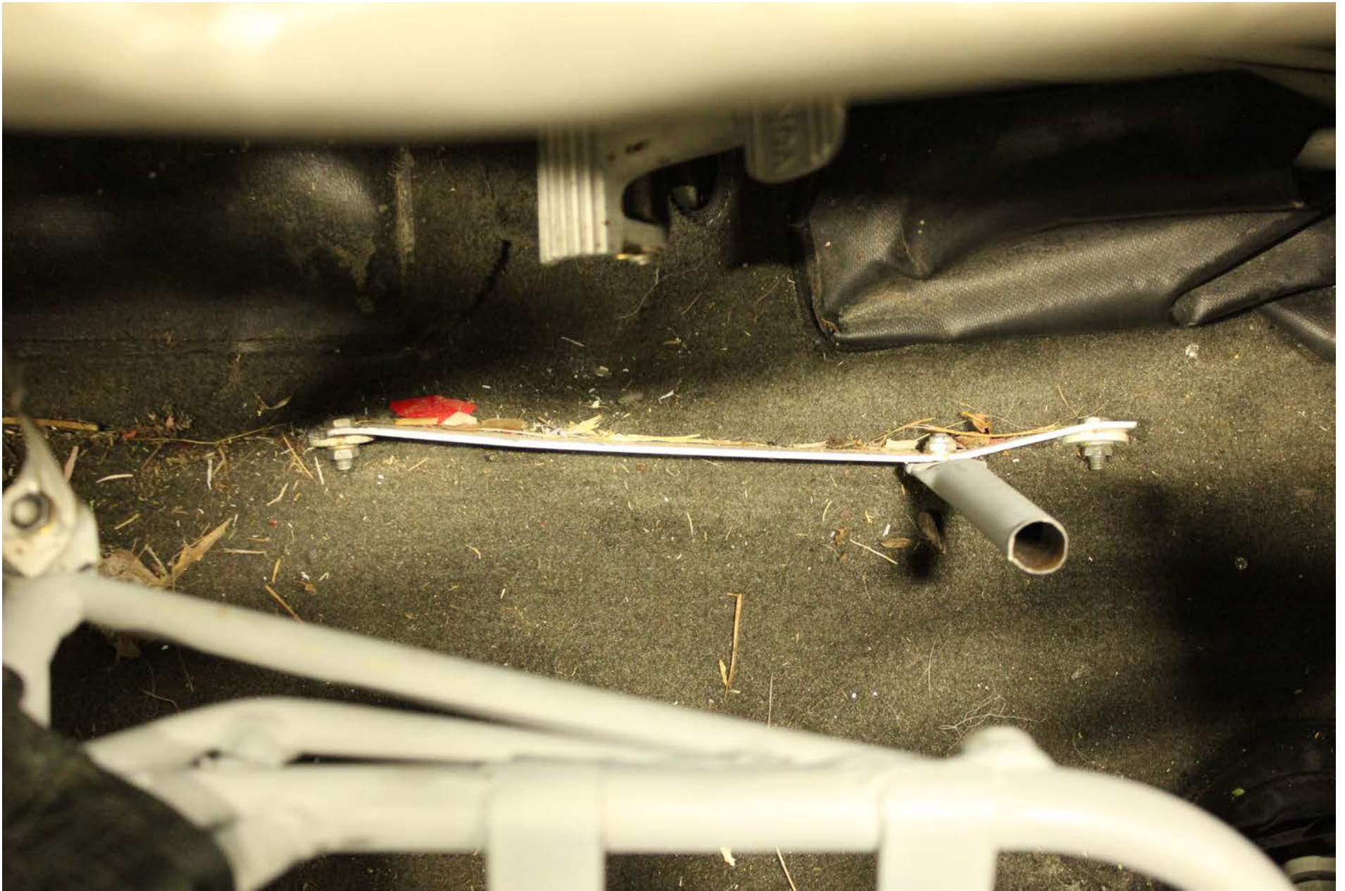
Photo 9 - Left side pilot seat leg fractures and modified bracket
