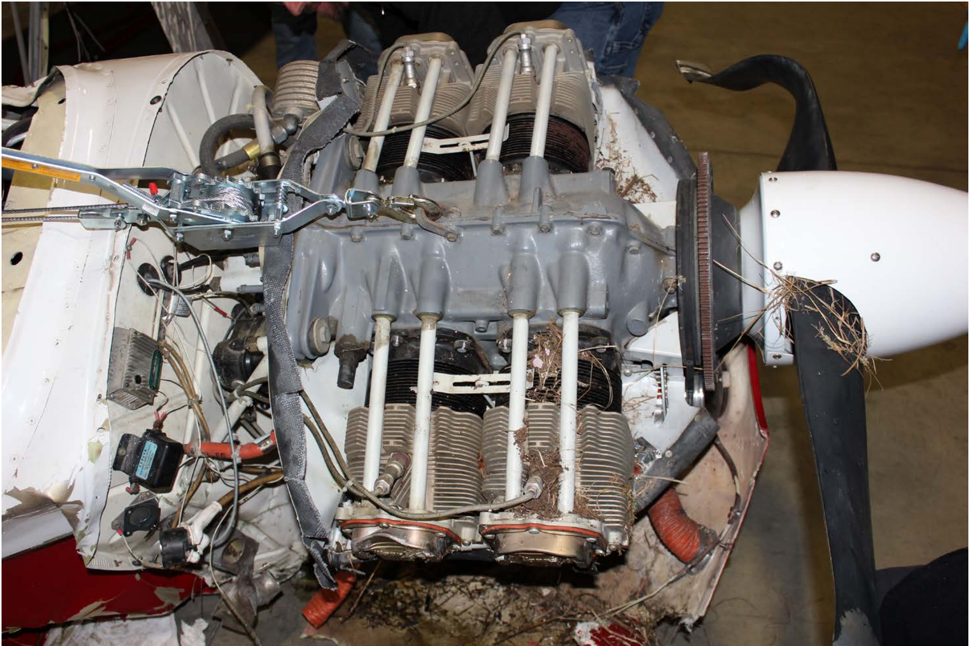
Photo 8 - Lycoming O-320 engine with right side damage
