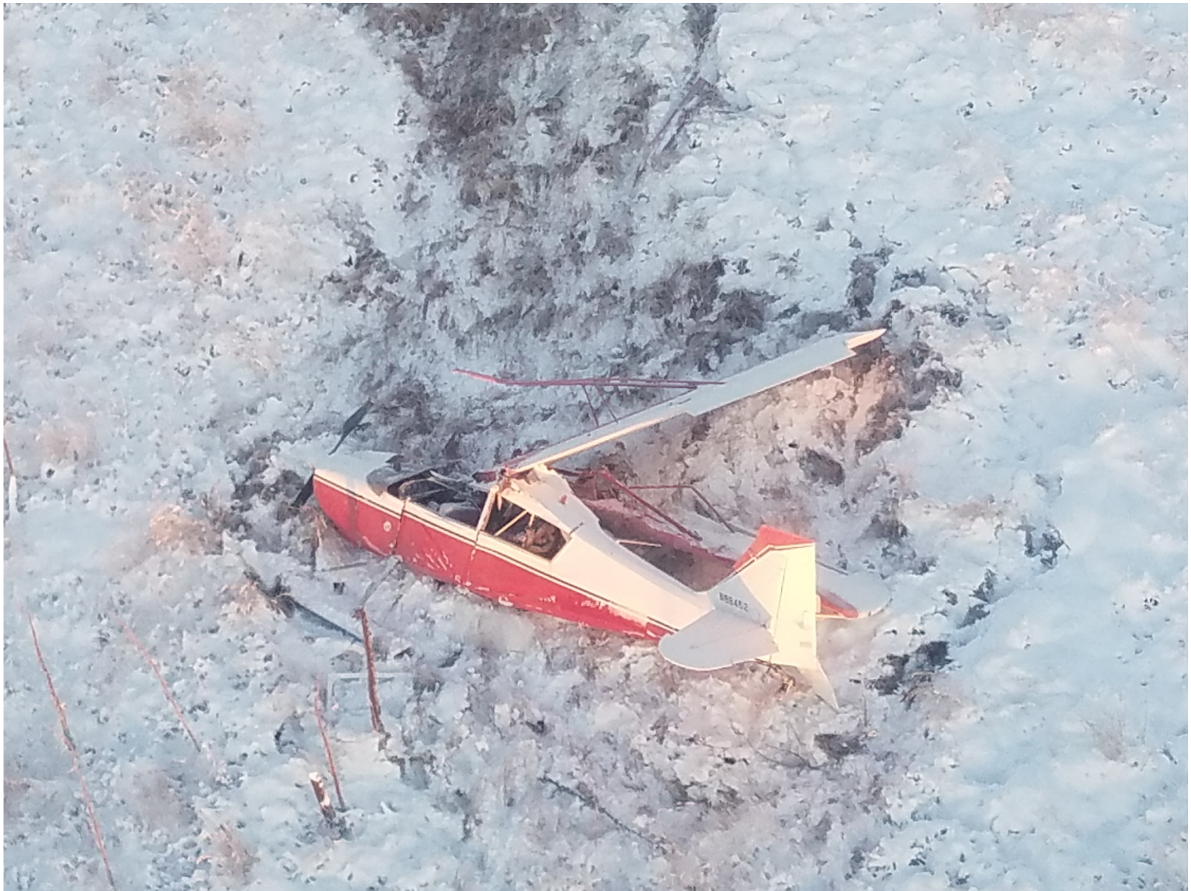
Photo 1 – N88452 Bellanca Citabria 7GCBC wreckage
