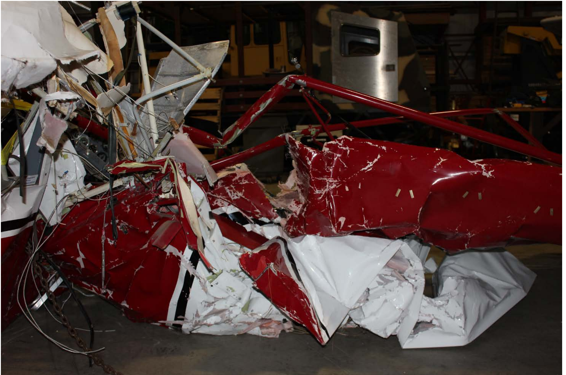
Photo 6 - Right wing root damage
