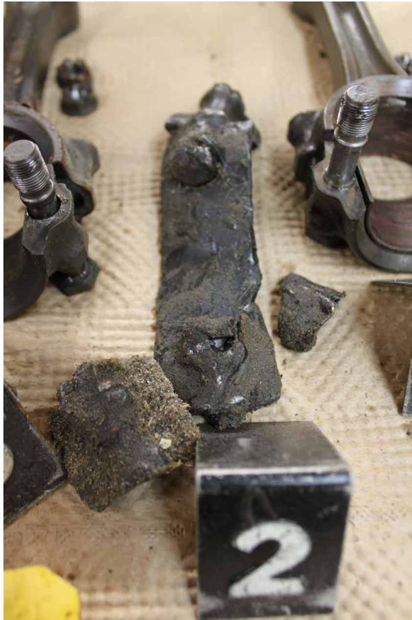
Photo 10 – Left engine number 2 connecting rod cap
