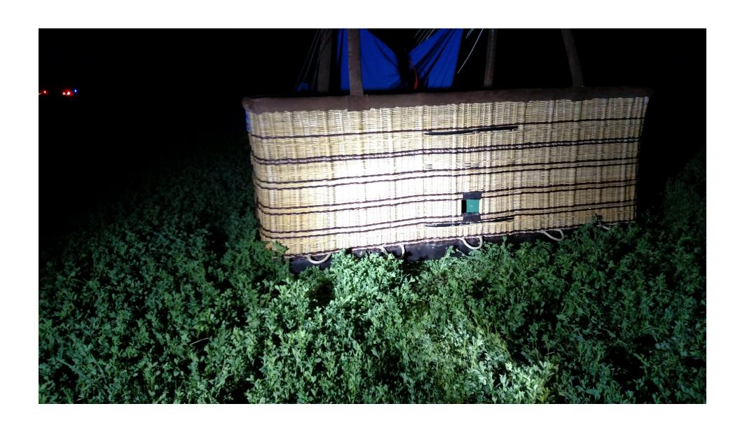
Photo 3 – View of entire side of basket showing the rope handles along the bottom. (Courtesy of FAA)
