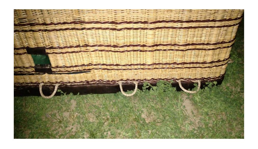
Photo 2 – Close up view of rope handles located on bottom of basket. (Courtesy of FAA)
