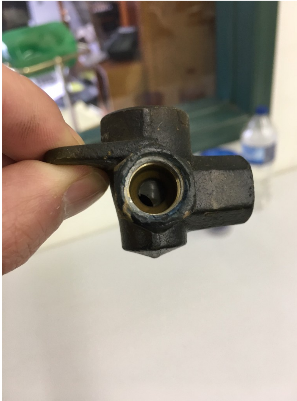
Photo 7 – Side View of Fuel Selector
