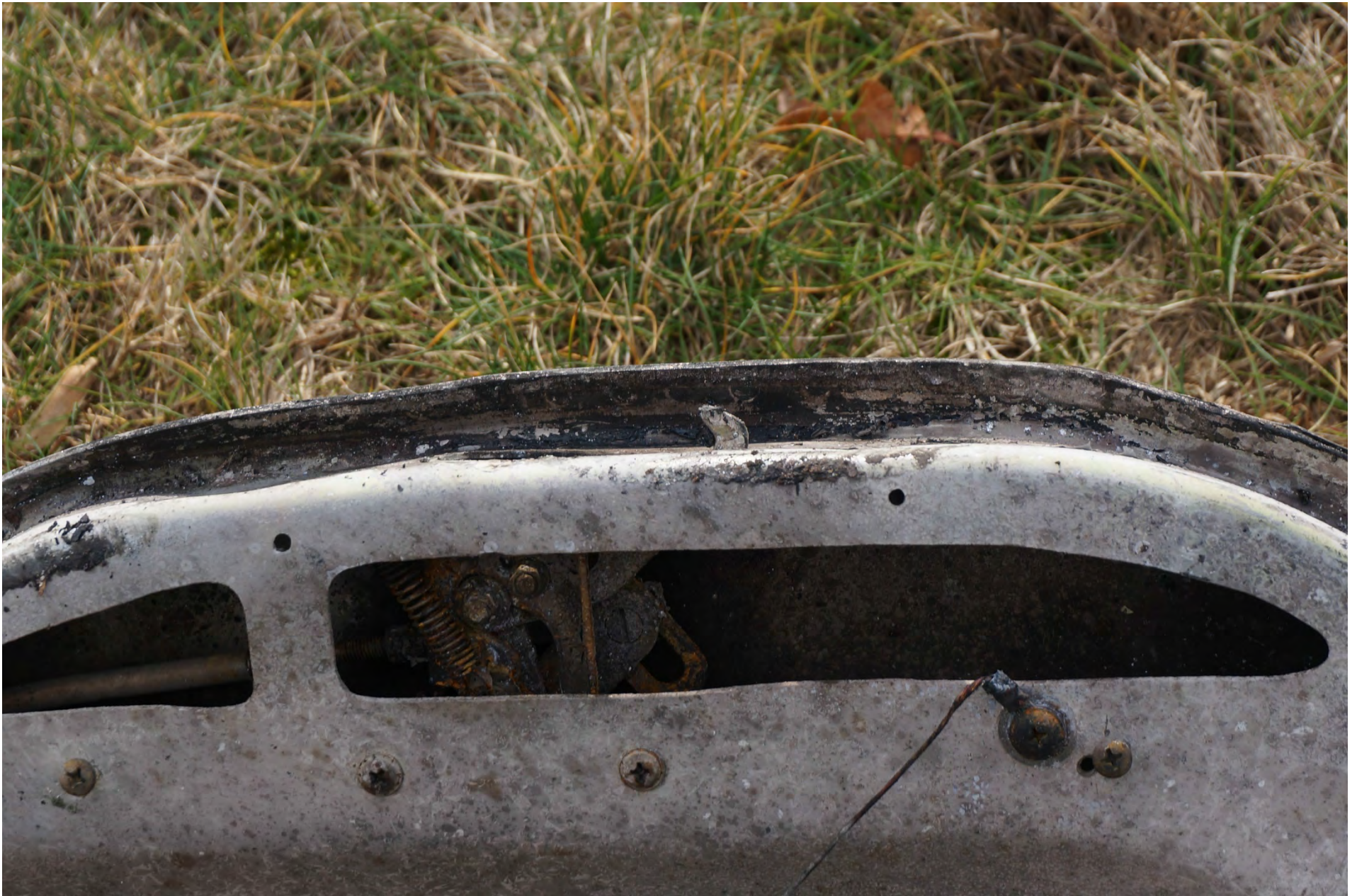
Photo 15 – Upper Door Latch After Removal of Door from Wreckage
