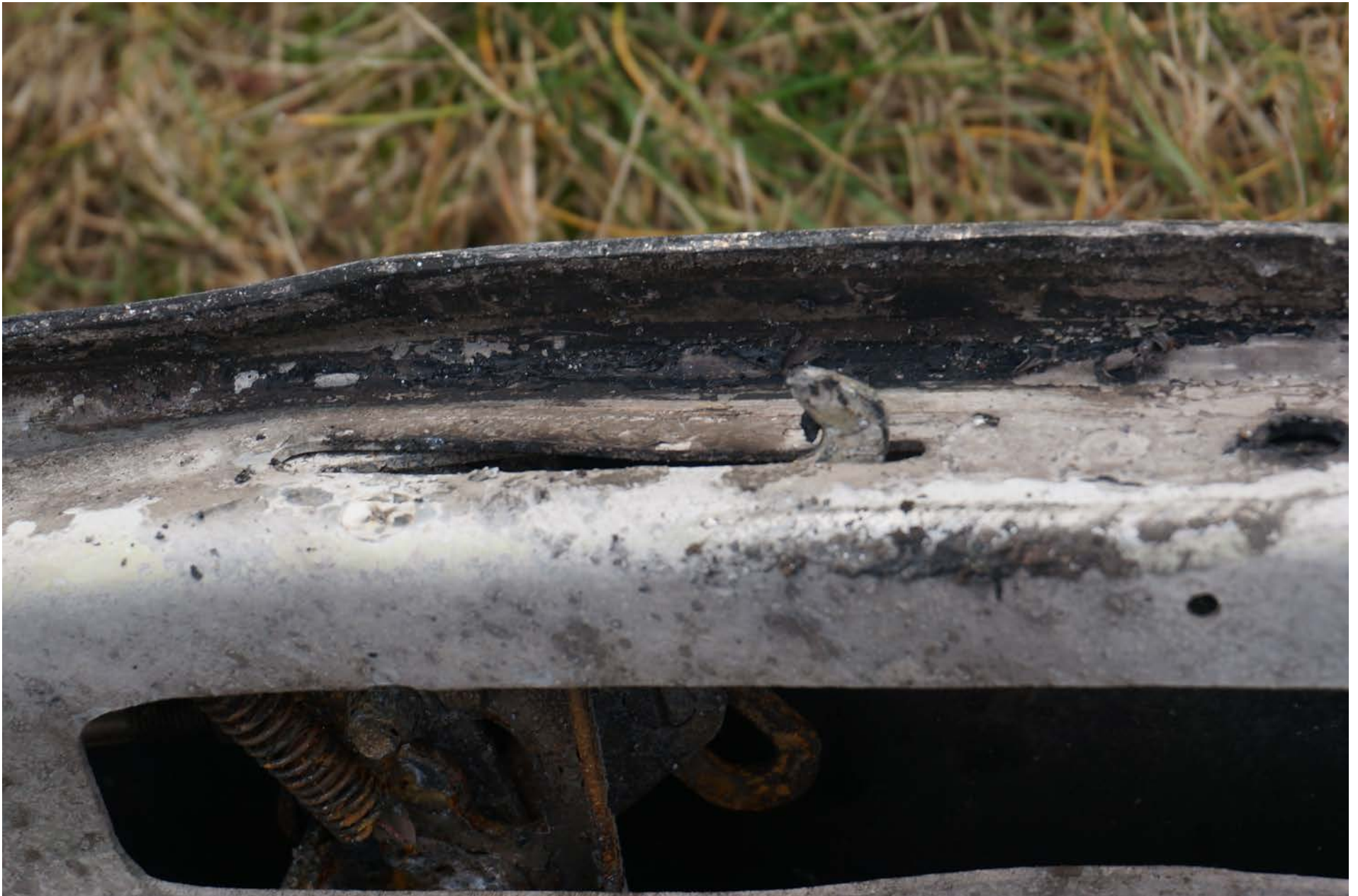
Photo 16 – Close Up of Upper Door Latch After Removal of Door from Wreckage
