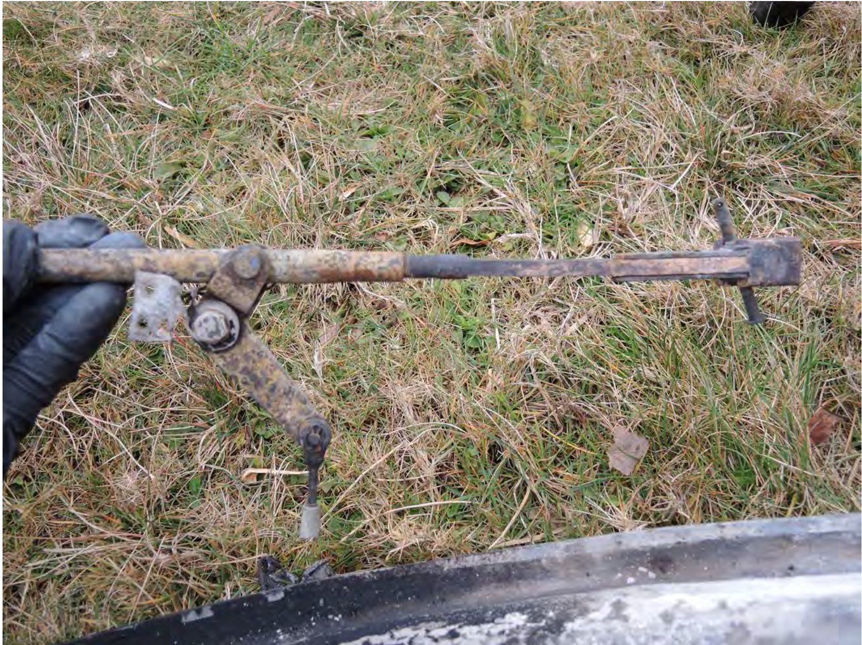
Photo 20 - Close Up of Aft End (Latch and Third Latch Point Bell Crank) – Courtesy of Textron Aviation
