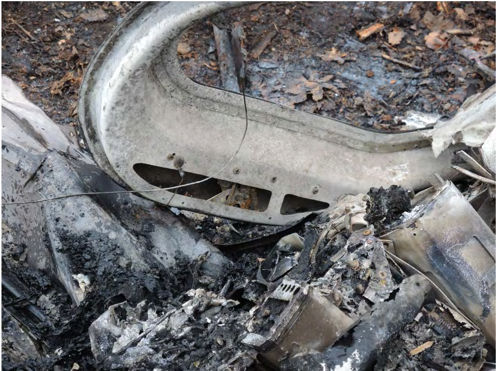
Photo 12 - Forward Cabin Door Upper Frame (Interior View) – Courtesy of Textron Aviation
