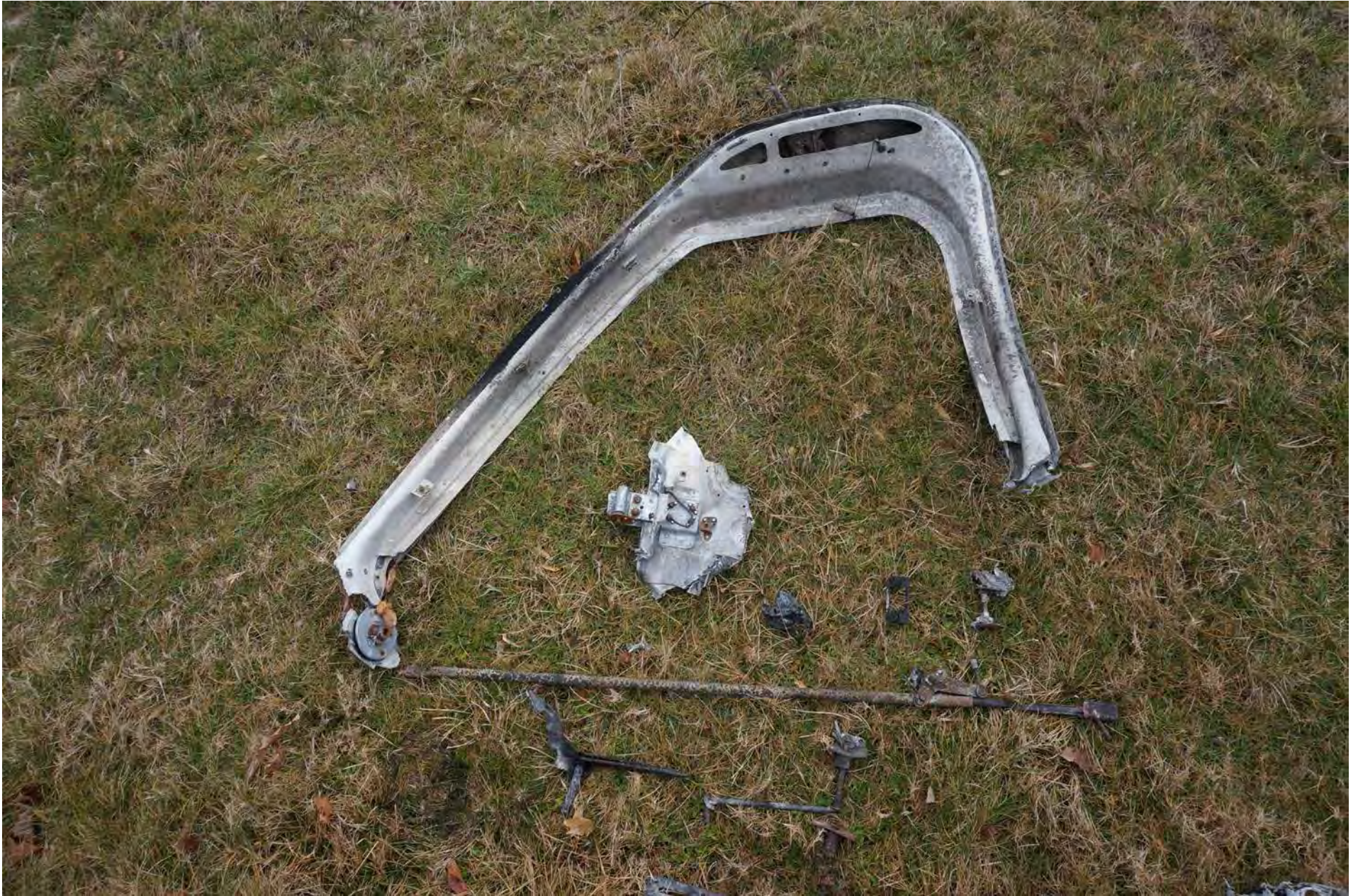
Photo 17 – Forward Cabin Door Locking Mechanism Components
