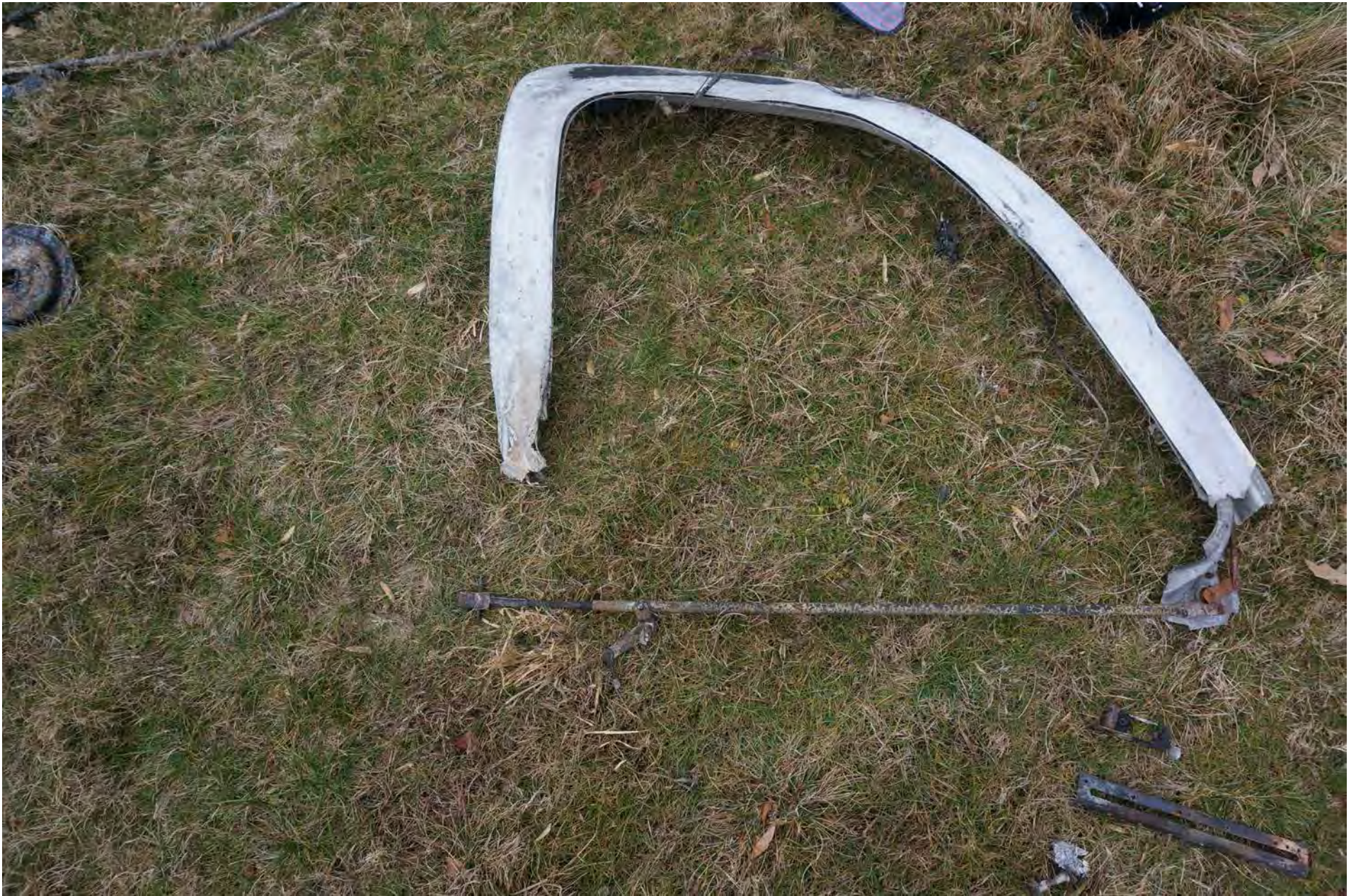
Photo 18 - Forward Cabin Door Locking Mechanism Components – Exterior View
