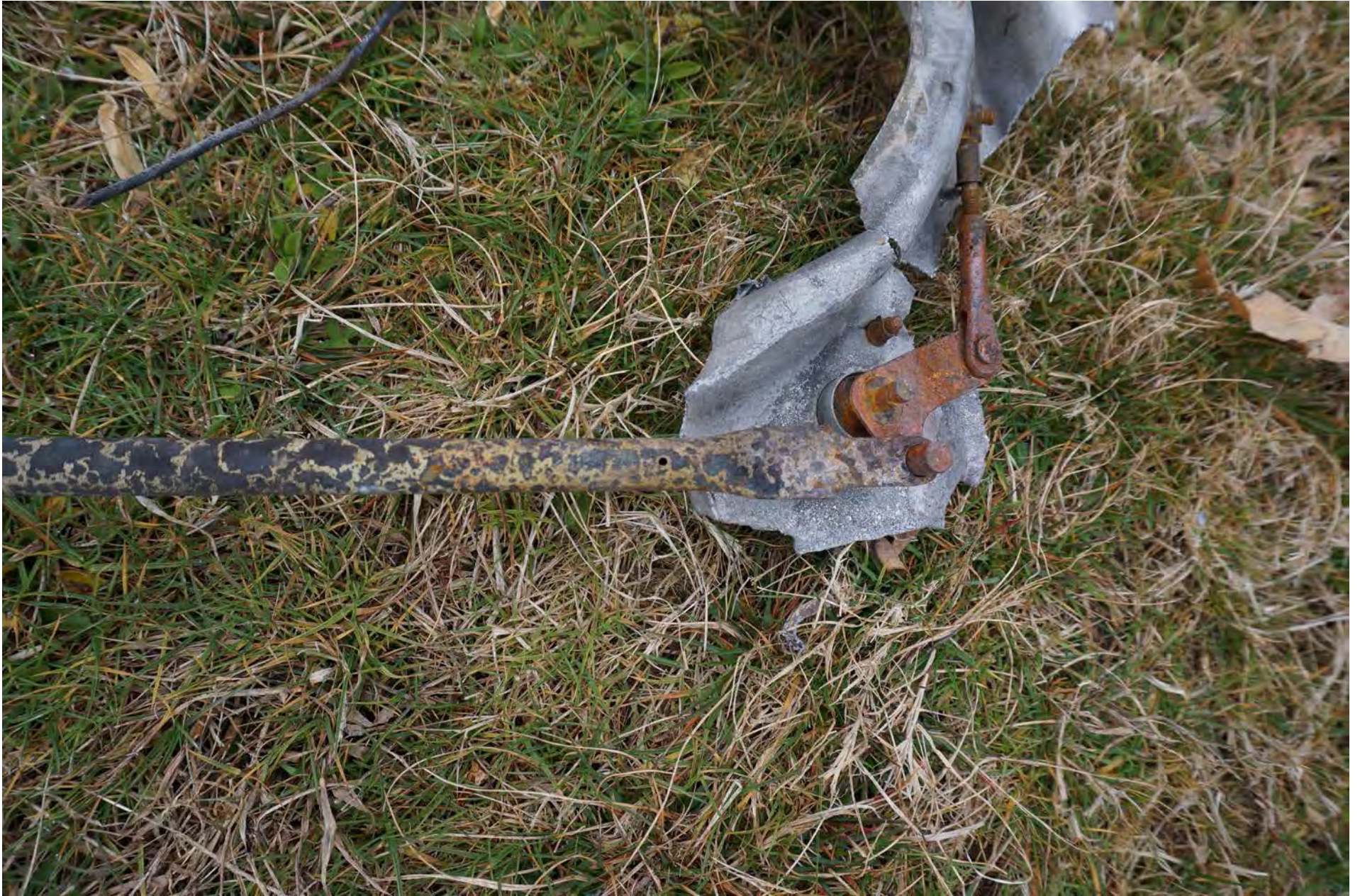
Photo 19 – Close Up of Forward End (Bell Crank Behind Interior Handle) of Locking Mechanism
