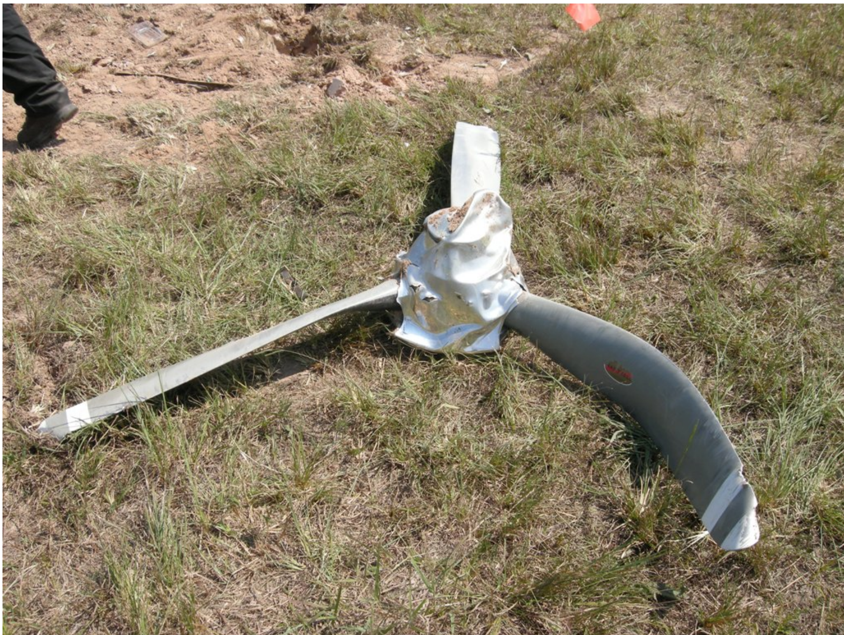
Photo 12 – Propeller from F33A (NTSB Photo)
