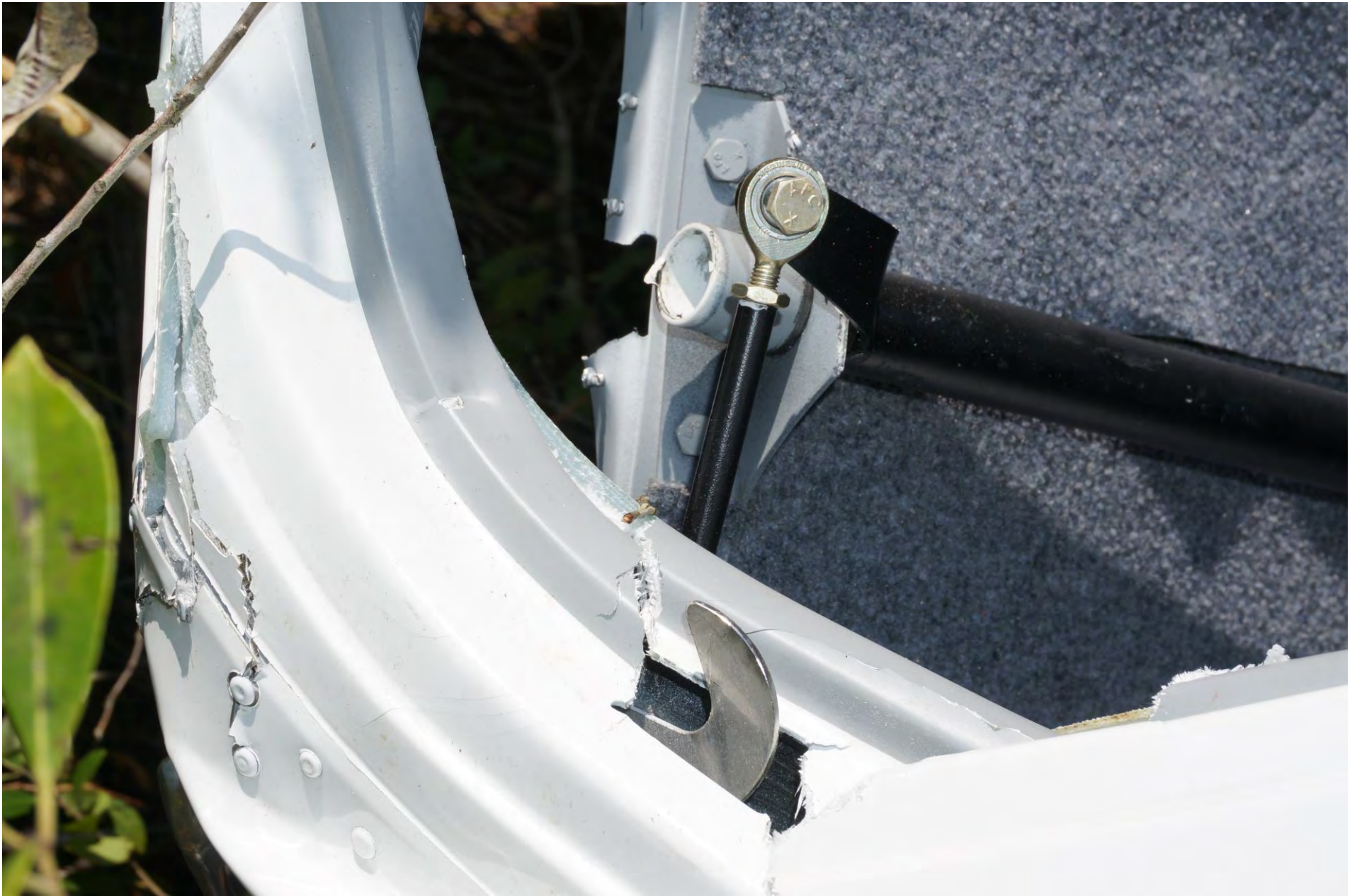
Photo 16 – Unlocked Left Side Canopy Latching Mechanism Hook
