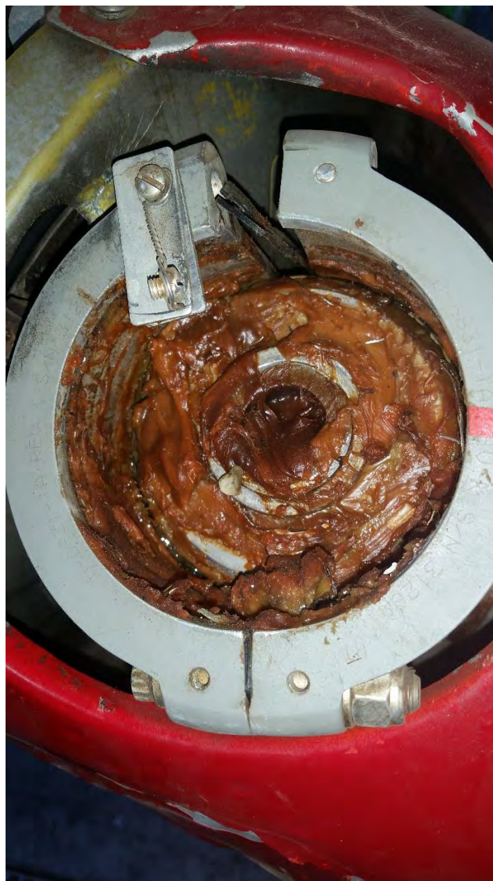
Photo 17 – Close Up of Blade Clamp After Recovery – Courtesy of FAA
