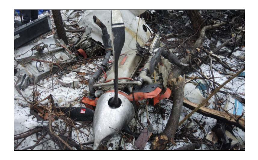
Photo 3 - Photo of engine with attached propeller near main wreckage.
