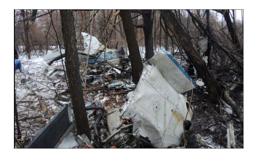
Photo 4 - Photo of second engine near main wreckage without propeller attached.
