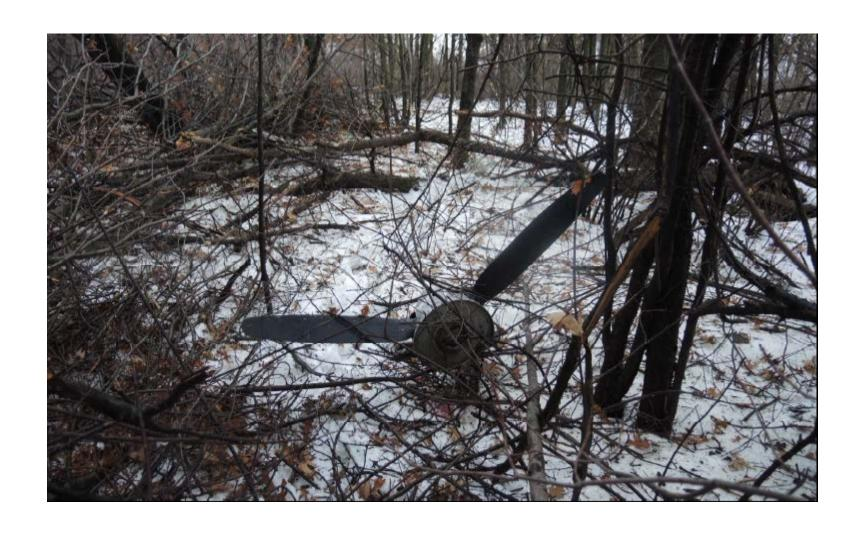
Photo 5 – Photo of second engine's detached propeller that was separated at the propeller hub.
