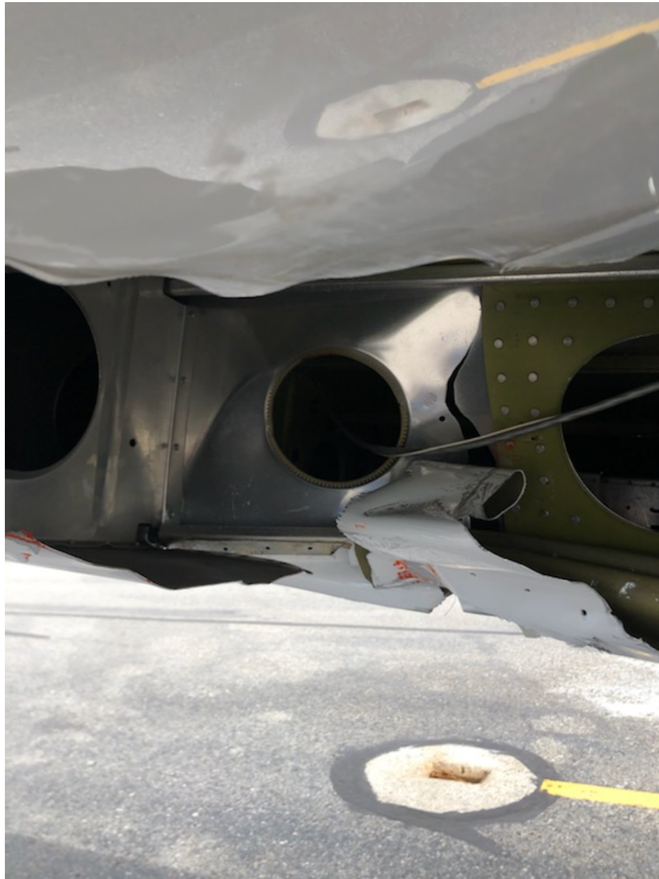
Photo 2 – right wing damage
