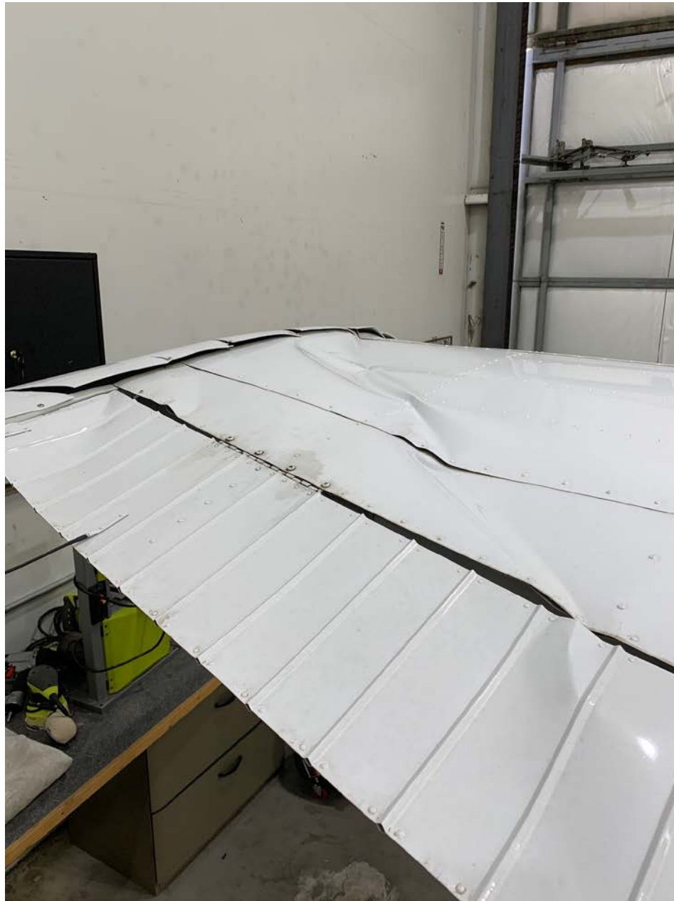
Photo 2 – photo of left outboard wing damage and left aileron
