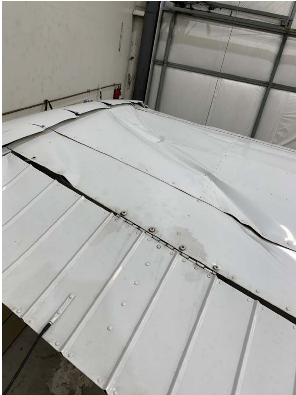
Photo 1 – photo of left outboard wing damage
