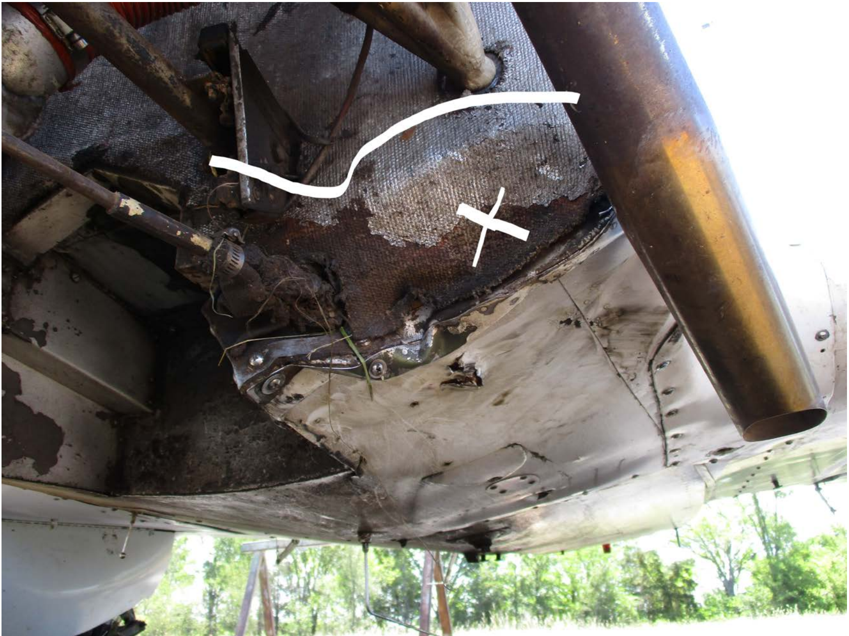
Photo 3 - Structural Damage to Underside of Front Fuselage
