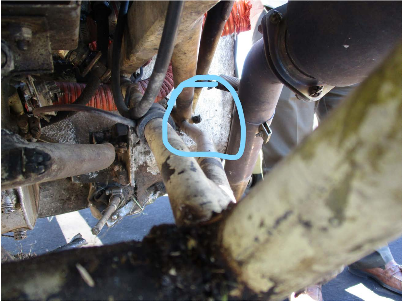
Photo 2 - Structural Damage to Underside of Front Fuselage
