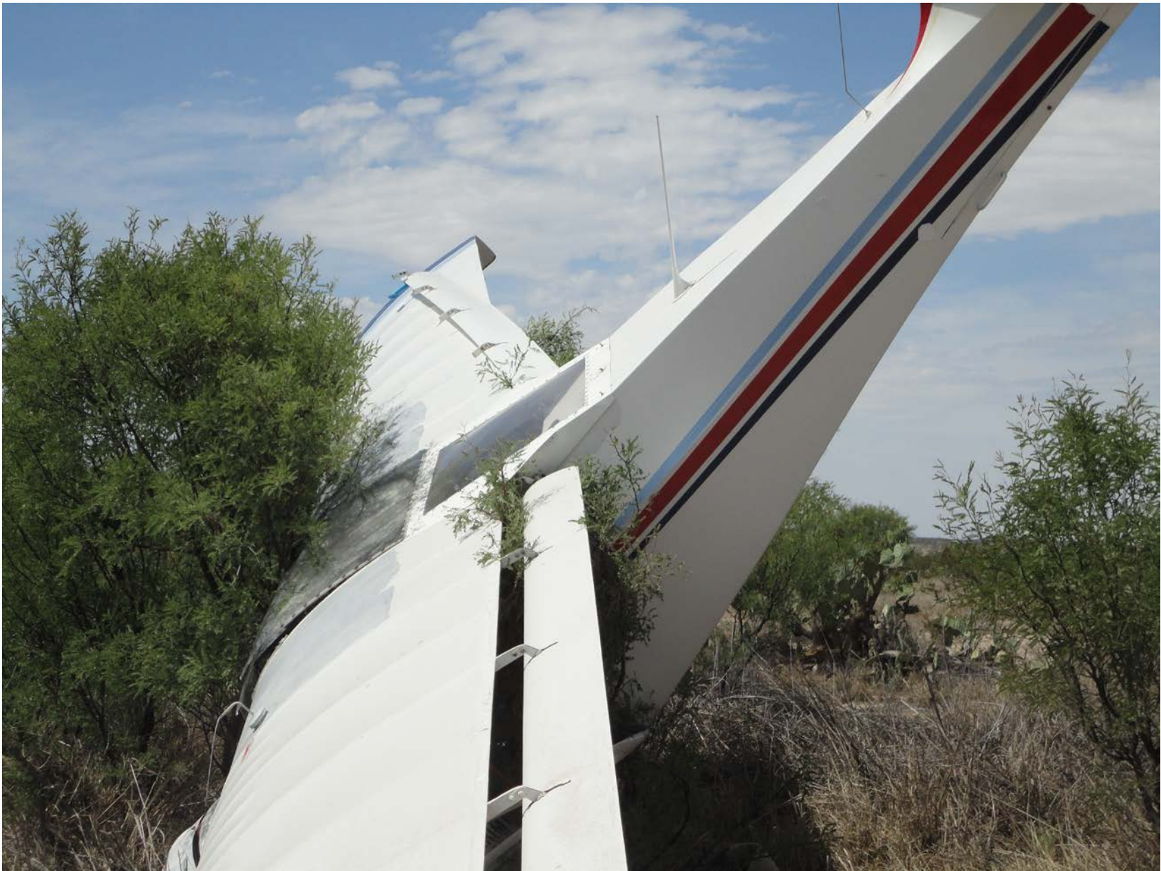
Photo 2 – Accident Site View of Wings and Damaged Flaperon Attach Points
