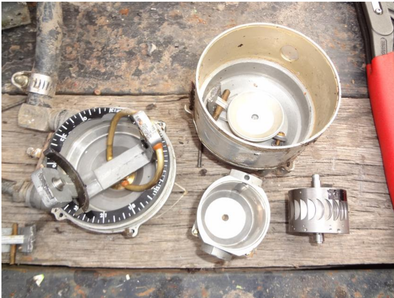
Photo 4 – Horizontal Situational Indicator (HSI) as Viewed (Post Disassembly)
