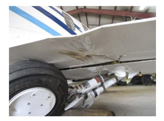
Photo 3 – View of Right Wing Damage (Courtesy of Insurance Adjuster)
