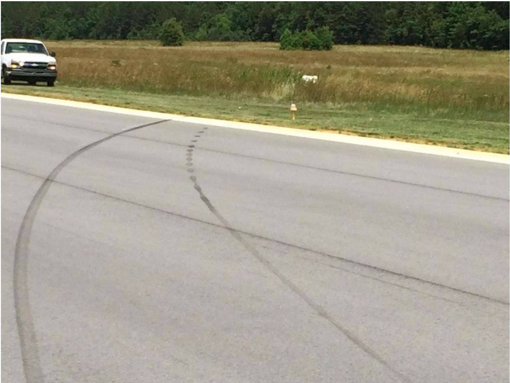
Photo 2 – Skid Marks Departing Runway (Courtesy FAA)
