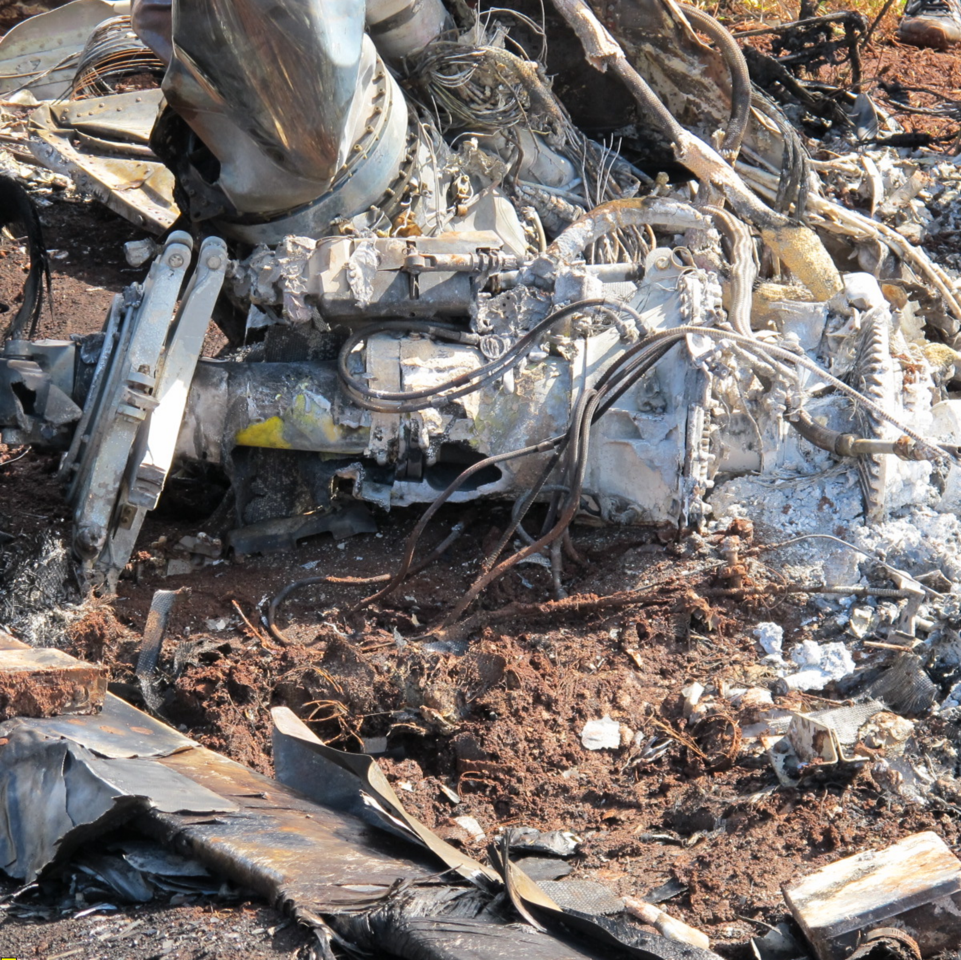
Photo 9. Main rotor gearbox and engine.
