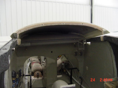
Photo 9. View From Forward Cockpit of the Installed Exemplar Canard
