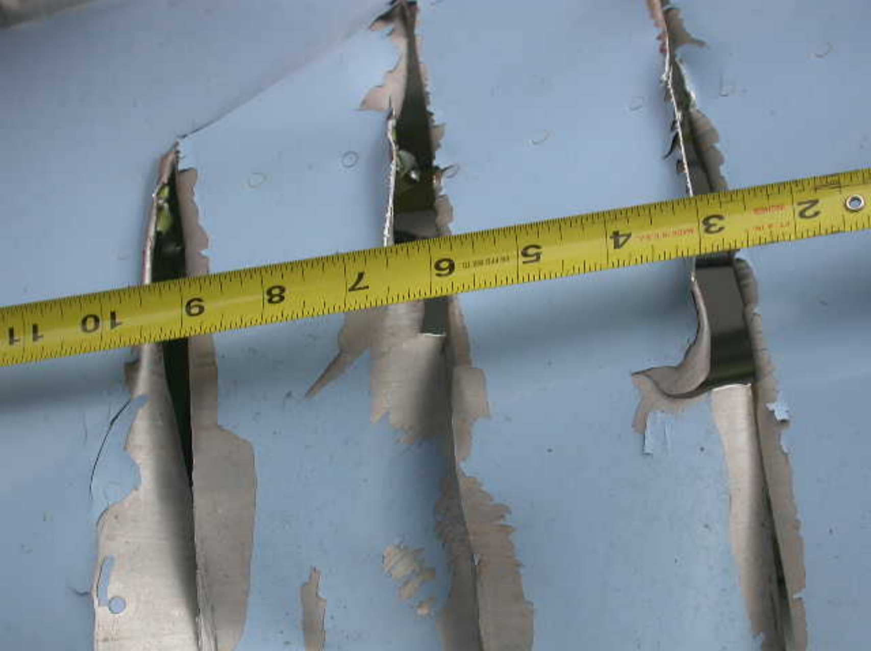
Photo 9. Measurement of Propeller Slashes on Fuselage
