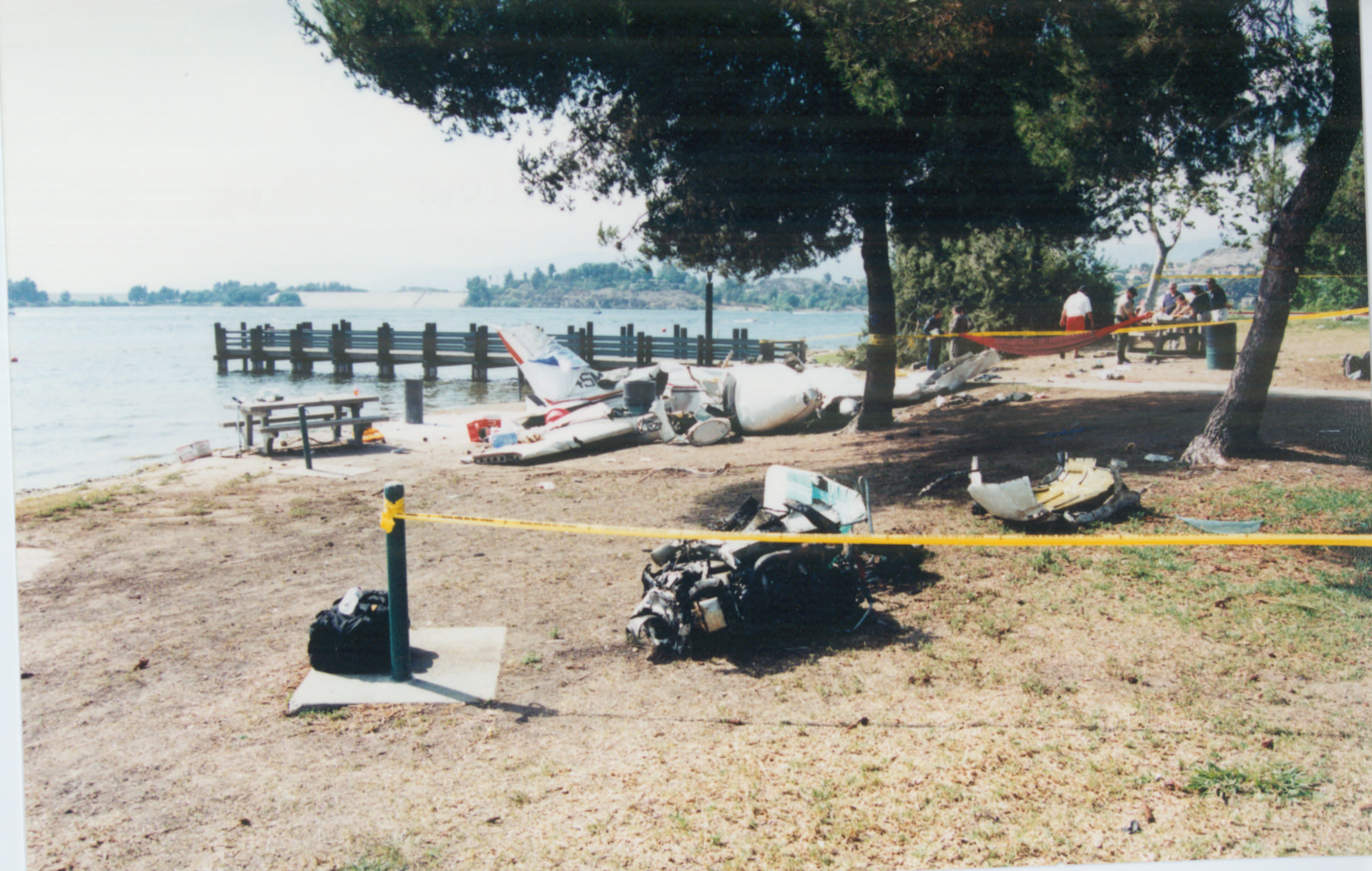
9-Main Wreckage with Right Engine in Foreground
